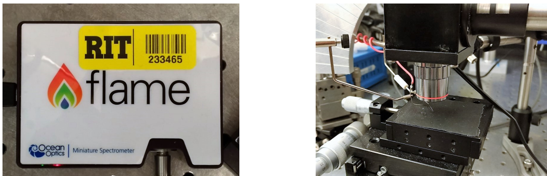
Figure 57. The electroluminescence measurement setup includes a rotating testing stage (right) and a Flame 200 nm – 850 nm spectrometer (left).
