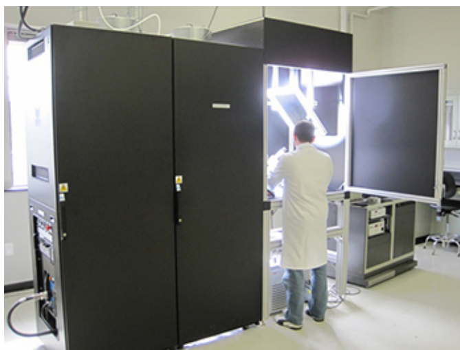
Figure 60. Parsian Mohseni is using the TS Space Systems two-zone close match solar simulator.
