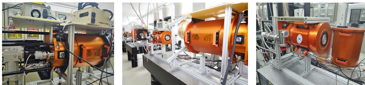
Figure 47. The four custom dewar test systems evaluate detectors in RIDL.
