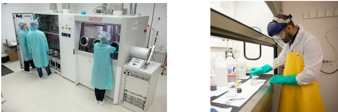
Figure 55. (left) PhD student Mohad Baboli loads a sample in the ALXTRON 3×2 Close Coupled Showerhead metal-organic chemical vapor deposition reactor, which is a part of the MOVPE. (right) PhD student Alireza Abrand is processing samples in the fume hood.
