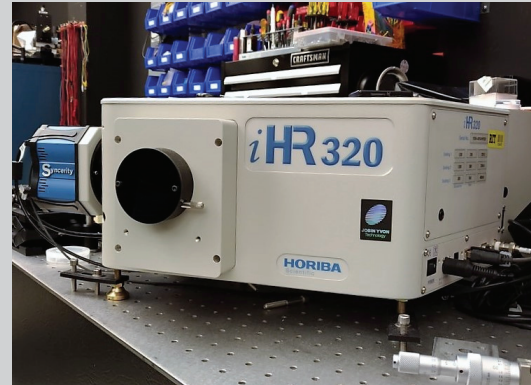
Figure 33. The Sincerity CCD Array detector (left) and the iHR320 spectrometer (right) are part of the photoluminescence system.
