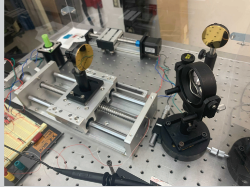
Figure 22. The current prototyped optical FTS (above) can determine the wavelengths of light traveling through in the system by changing the position of the mirror on the stage and observing the voltages from a detector.
