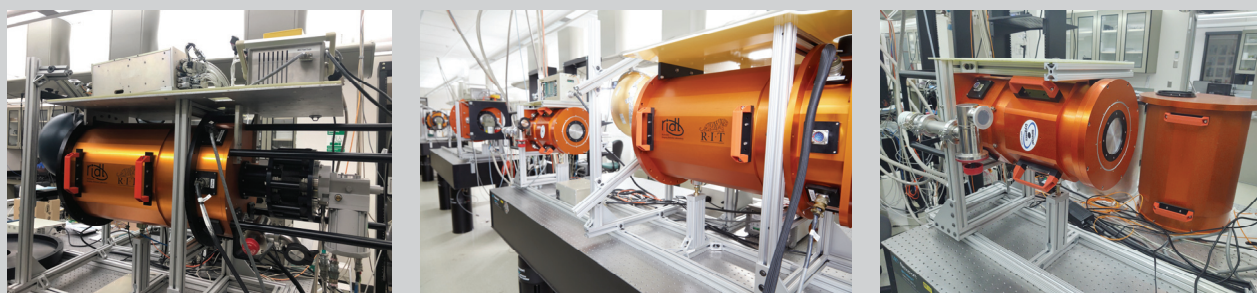
Figure 30. Staff and students use the four custom dewar test systems to evaluate detectors in RIDL.
