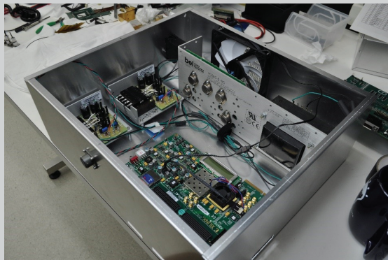
Figure 23. Pictured above is the Warm Electronics Board Assembled for the SAT QIS Project.
