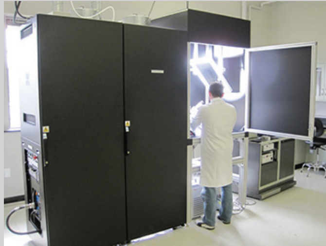
Figure 43. Parsian Mohseni is using the TS Space Systems two-zone close match solar simulator.
