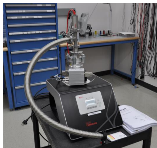
Figure 38. (left) A team of undergraduate students are using function generators, oscilloscopes, and FPGA based control boards to develop an image sensor readout package that will fly on a suborbital platform. (right) A new Oerlikon Leybold Turbolab turbo-molecular pumping station was procured during the past year.
