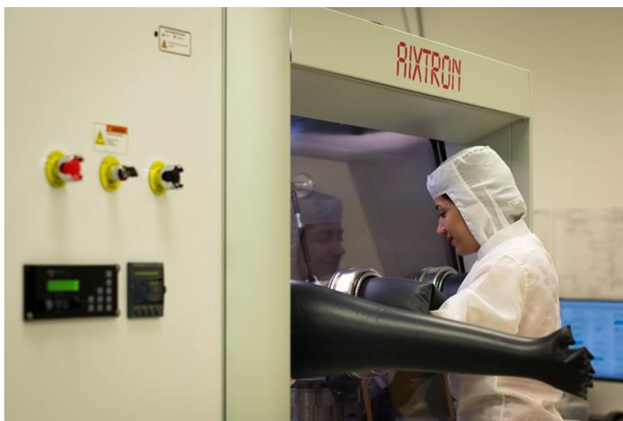
Figure 21. Mohad is seen here loading a sample in the AIXTRON 3x2 Close Coupled Showerhead metal-organic chemical vapor deposition (MOCVD; RIT NanoPower Research Laboratories) reactor for crystal growth of III-V semiconductor nanowires.
