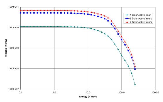
Figure 16: Shielded solar proton energy spectra for 100 mils aluminum 95% confidence level
