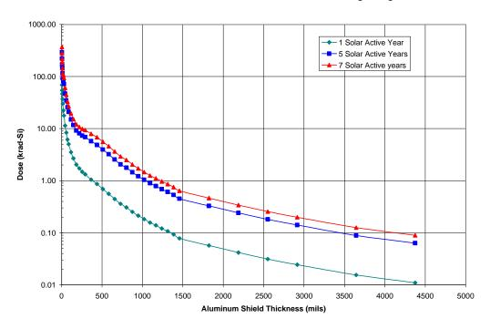
Figure 17: Total ionizing dose from solar proton events for 1, 5, and 7 solar active years is presented.
