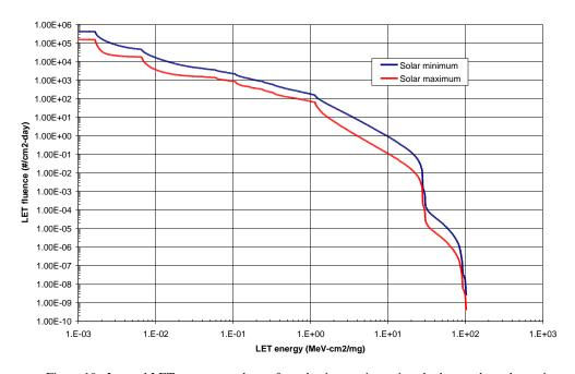
Figure 19: Integral LET spectra are shown for galactic cosmic ray ions hydrogen through uranium.
