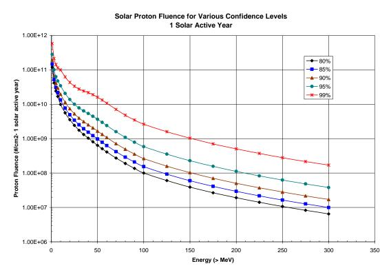
Figure 9: Solar proton fluences for 1 solar active year are presented for various confidence levels.
