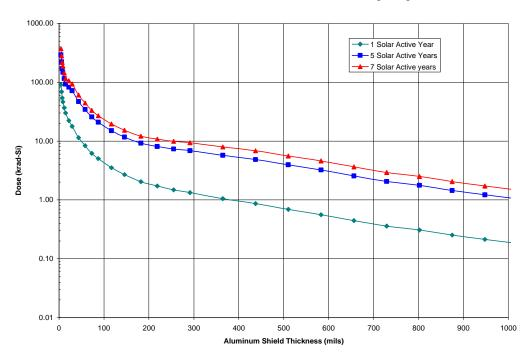
Figure 18: Total ionizing dose from solar proton events for 1, 5, and 7 solar active years is presented.
