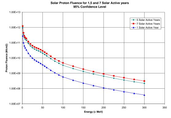
Figure 12: Solar proton fluences for a 95% confidence level are presented for 1, 5, and 7 solar active years.
