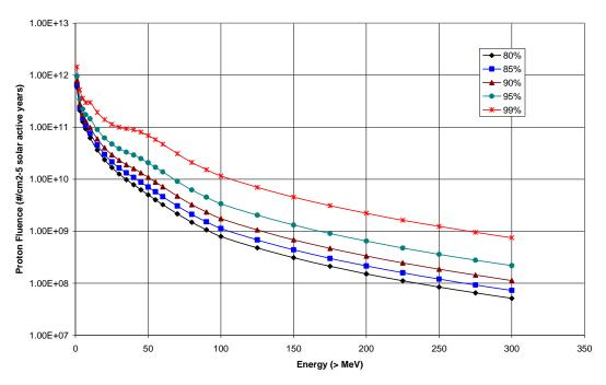
Figure 10: Solar proton fluences for 5 solar active years are presented for various confidence levels.
