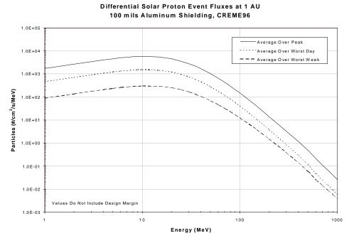
Figure 21: Solar proton fluxes for single event effects evaluation.
