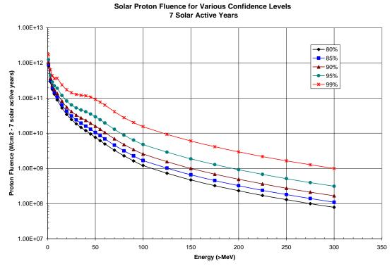
Figure 11: Solar proton fluences for 7 solar active years are presented for various confidence levels.
