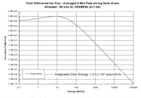
Figure 23: Total differential fluence of all predicted solar particles based on the October 1989 event
