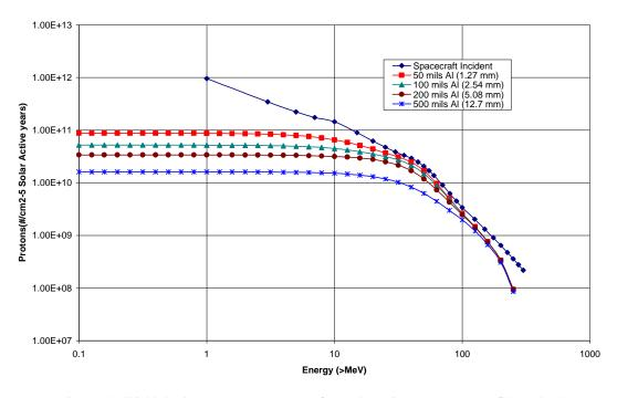
Figure 14: Shielded solar proton energy spectra for 5 solar active years, 95% confidence level.
