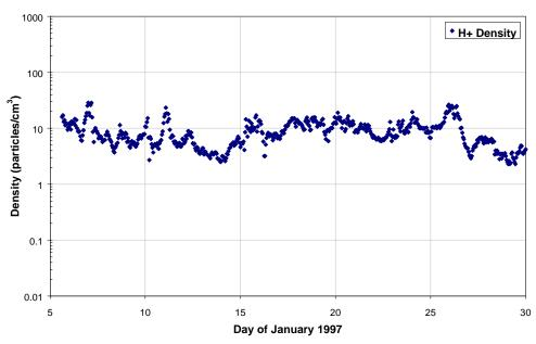
Figure 4: A sampling of the solar wind density as measured by the SOHO spacecraft.
