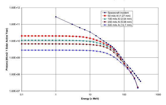
Figure 13: Shielded solar proton energy spectra for 1 solar active year, 95% confidence level.
