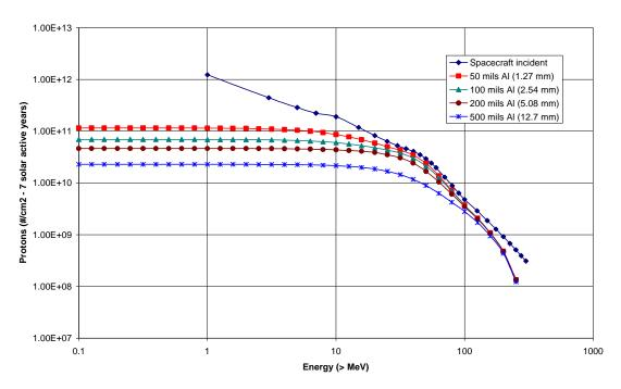
Figure 15: Shielded solar proton energy spectra for 7 solar active years, 95% confidence level.
