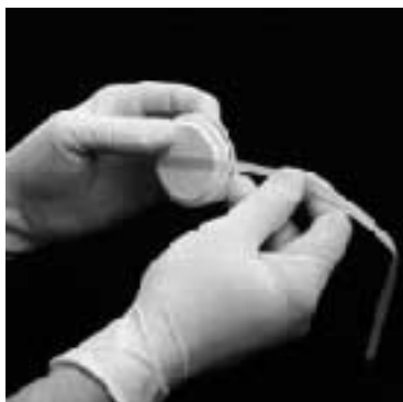
Figure 2. Attaching a cover over an optical coated surface.
