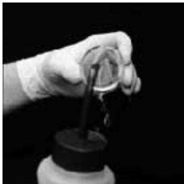
Figure 1. Flushing the optical device with Vertrel XF or Asahiklin AK-225.
