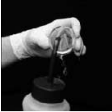
Figure 1. Flushing the optical filter with Vertrel XF or Asahiklin AK-225.
