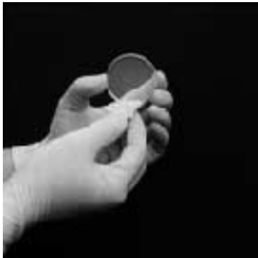
Figure 2. Blotting the lower edge of the filter without contacting the coated surface.
