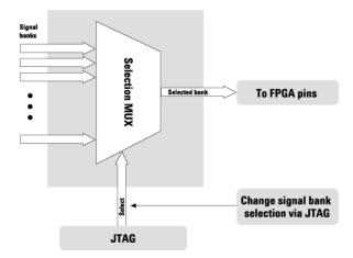
The Altera LAI core provides a multiplexer for selecting the signals that are output to FPGA debug pins. Core parameters determine the number of signals per bank and the number of banks.
