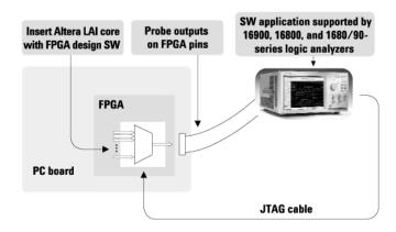
Create a time-saving FPGA measurement system. Insert an Altera LAI (Logic Analyzer Interface) core into your FPGA design. With the application running on your logic analyzer via JTAG, you control which group of internal signals to measure.
