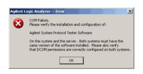
The "Agilent System Protocol Tester" software must be installed on the system where the *Agilent Logic Analyzer* application is running and on the system that is being used as the protocol analyzer server. It can be installed on the logic analysis system frame if you want to run both applications there.
