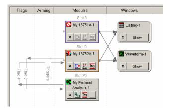
Note that the trigger icon and menu items are enabled – this shows the connection is active and lets you change the cross-triggering or trigger deskew setup.
