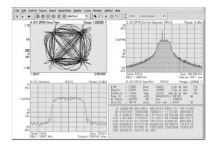
Figure 4 Agilent 89601A vector signal analysis software
