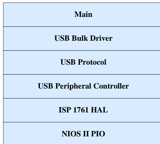
Figure 5.7. Software Stack of the USB-Device Demonstration
