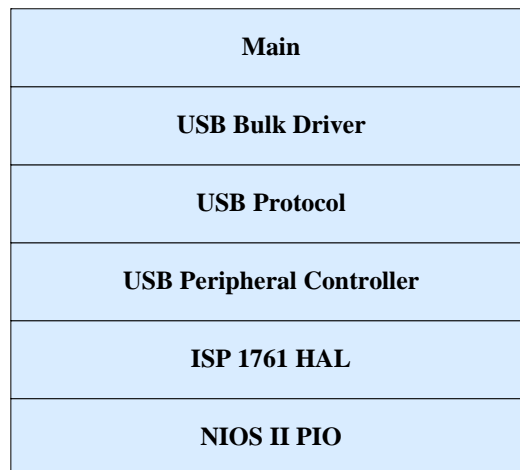
Figure 5.7. Software Stack of the USB-Device Demonstration
