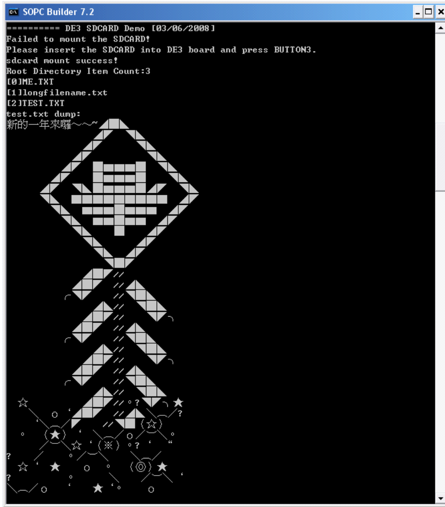
Figure 5.14. Display SD Card Information for the SD Card Demonstration
