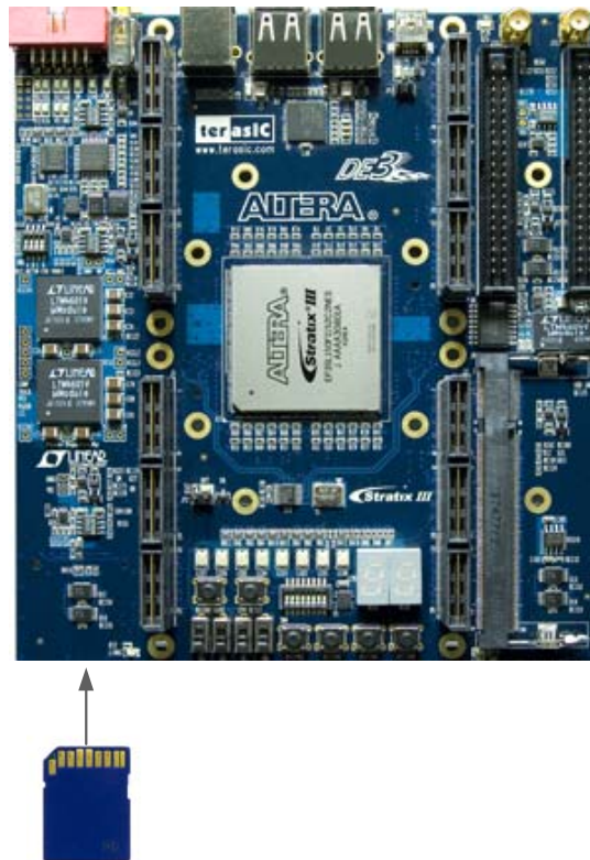
Figure 5.13. Insert SD Card for the SD-Card Demonstration
