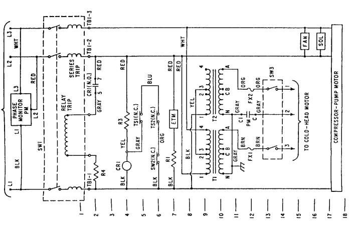
Figure B.1 Electrical schematic for the Model 1020R compressor P/N 8031023G001 or
