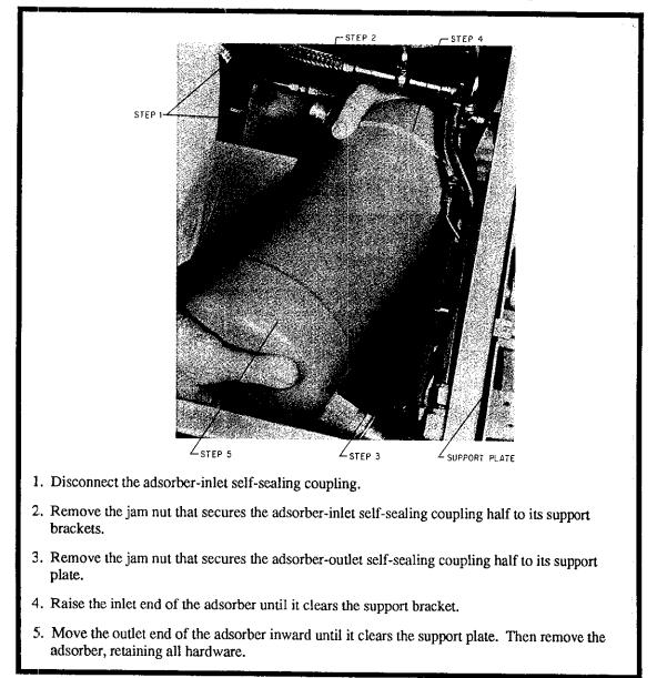
Figure 5.2 Removing the adsorber from the Model 1020R Compressor
