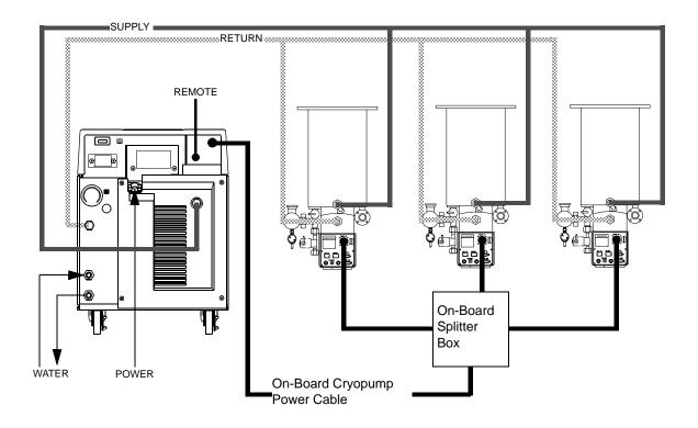
Figure 1-5: 9600 Compressor Connected to Multiple On-Board Cryopumps
