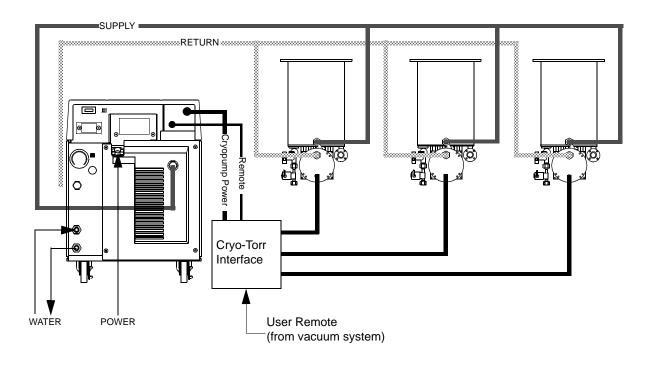
**Figure 3-9: Multiple Cryo-Torr Cryopump Installation**
