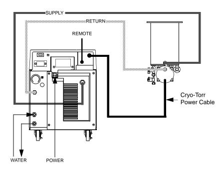
Figure 3-5: Single Cryo-Torr Cryopump Installation
