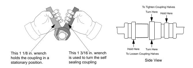
Figure 5-1: Disconnecting Self Sealing Couplings
