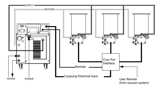
Figure 1-6: 9600 Compressor Connected to Multiple Cryo-Torr Cryopumps
