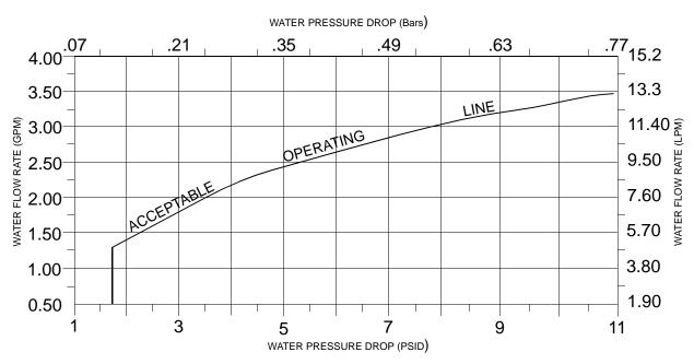
**NOTE:** Figure 1-3 defines the water flow rate through the Compressor as a function of the pressure drop from water inlet to water outlet. You must provide the correct pressure drop in your water supply system to ensure that the water flow condition meets the requirements specified in Table 1-3.
