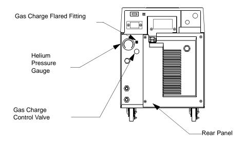
Figure 5-3: Helium Pressure Control Components
