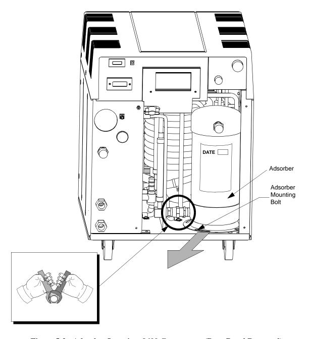
Figure 5-2: Adsorber Location, 9600 Compressor (Rear Panel Removed)
