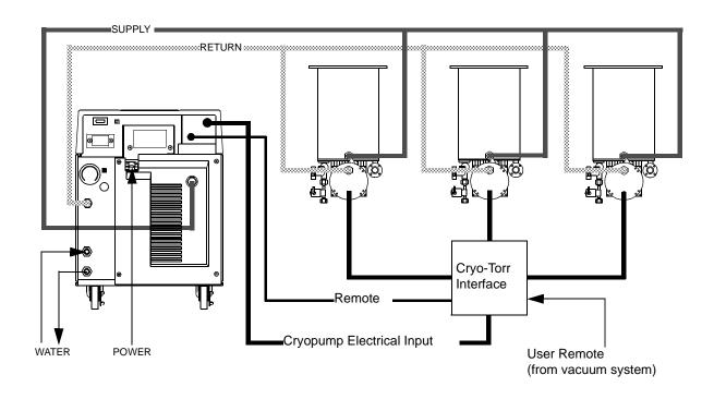
Figure 3-8: Multiple Cryo-Torr Cryopump Installation
