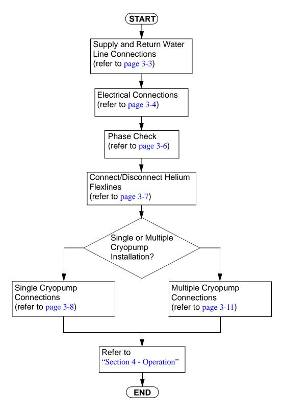
Figure 3-1: 9600 Compressor Installation Flowchart
