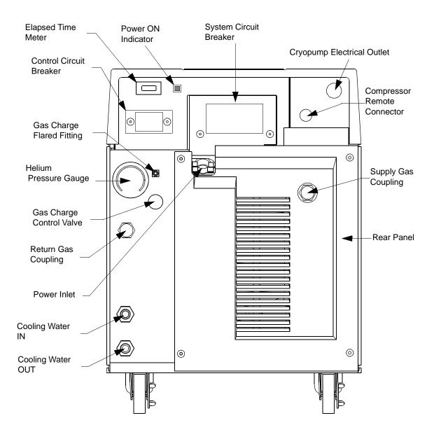
Figure 1-4: 9600 Compressor Rear View Component Locations
