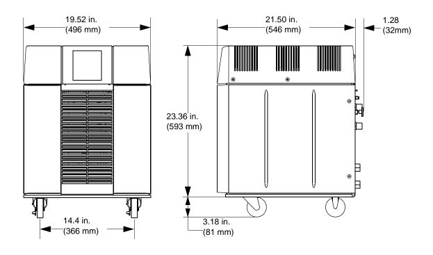
**Figure 1-2: 9600 Compressor Dimensions**
