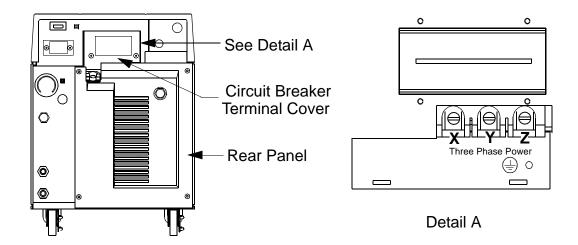
**NOTE:** Use a slotted screwdriver which is capable of holding a screw when performing steps 9 and 10.
