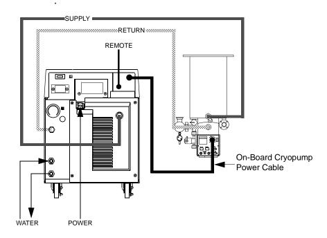
Figure 3-4: Single On-Board Cryopump Connections
