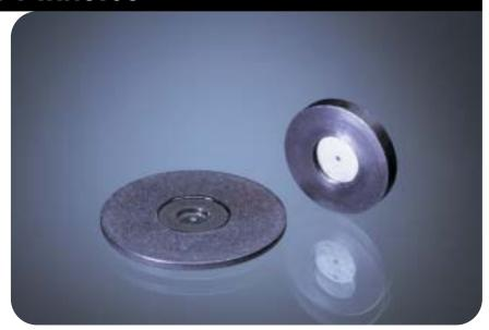
Ealing UV/Visible Laser Pinholes are specifically designed to work with most UV and visible lasers, such as Ar Ion, HeNe, or Kr. They are made from a specially developed molybdenum alloy, allowing for high power CW usage. Typical applications include spatial filtering and holography. They are supplied in either 16mm or 25mm diameter mounts.
