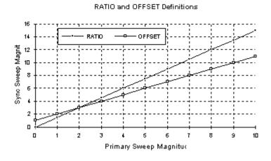
Figure 2-28: Synchronous Sweep "Ratio" and "Offset" Definitions.
