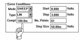
Figure 2-32: Designating a Measurement Compliance
