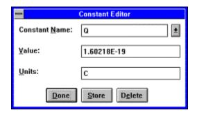
**Figure 5-7:** The Constant Editor Dialogue Box Provides the Capability to Edit, Add, or Delete Constants from the Constants List Box.
