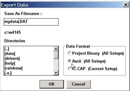
Figure 7-6: How to Export a Project File in ASCII Format
