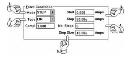
Figure 2-30: How to Source a Step Signal
