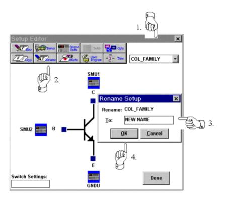
Figure 2-21: How to Rename a Test Setup.
