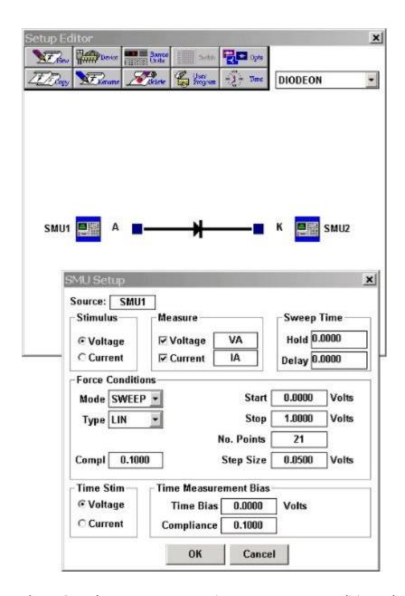
**Figure 2-1:** The test setup stores instrument setup conditions, documents the instrument/DUT connections, and stores what data is returned and how it is labeled.
