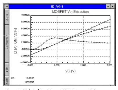
Figure 5-8: Plot of ID, GM, and GMFIT versus VG.
