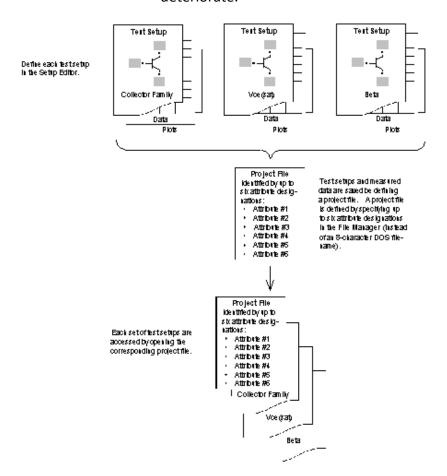
**Figure 2-2:** One or More Test Setups make up a Single Project File. A Test Setup is only Accessible from the Project File in which it was Created.
