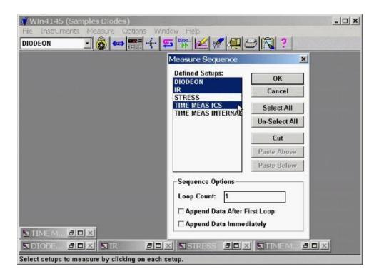
**Figure 4-5:** How to Define a Test Setup Sequence.
