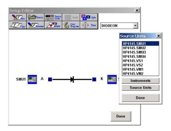
**Figure 2-8:** How to Designate a Connection Between the Instrument and the DUT.
