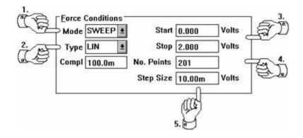
Figure 2-27: How to Source a Sweep Signal
