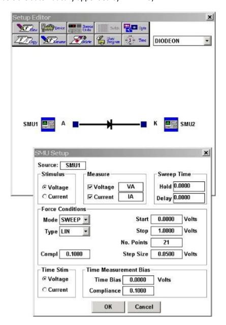
**Figure 1-2:** The test setup stores instrument setup conditions, documents the instrument/DUT connections, stores what data is returned and how it is labeled.
