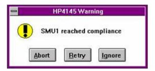
**Figure 2-24:** Win4145 Reports Compliance Events if the Report Compliance Switch is Selected in the Mainframe Setup Dialogue Box.
