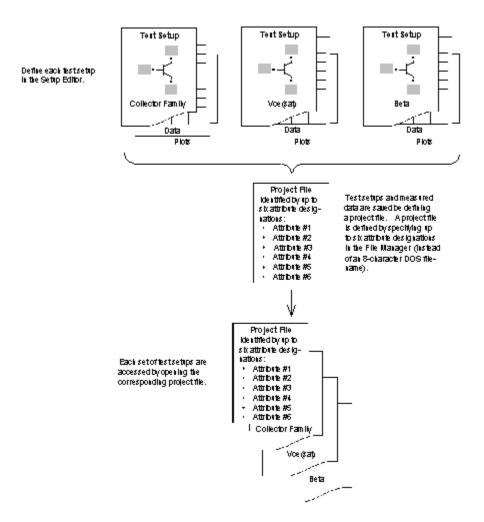
**Figure 1-4:** One or More Test Setups make up a Single Project File. A Test Setup is only Accessible from the Project File or Temp File in which it was created.
