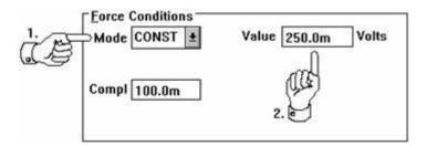
Figure 2-31: How to Force a Constant Signal
