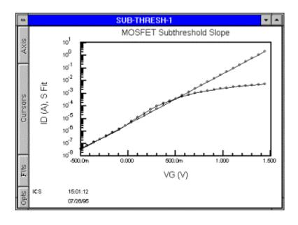
Figure 5-10: Plot of ID and S Fit versus VG.
