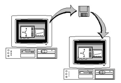
**Figure 7-3:** The Binary Export Function Provides the Capability to Copy Project Files from one Machine to Another.
