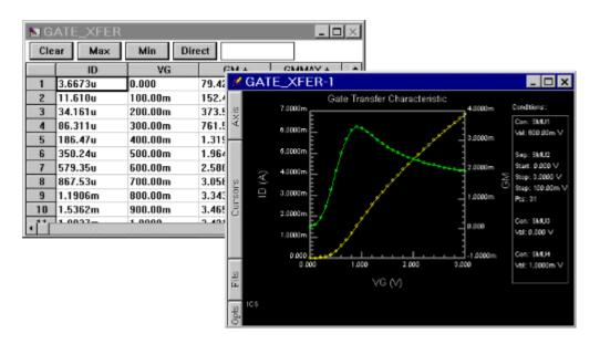
**Figure 5-5:** The Transform Editor provides the User with the Capability to Define Data Vectors that are Functions of Measured Data.
