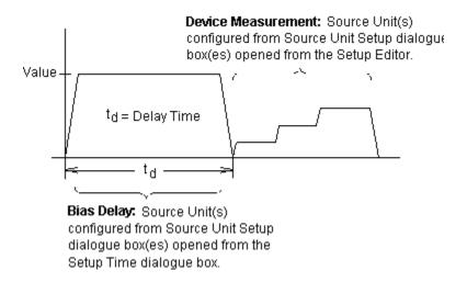
**Figure 2-13:** An Example of a Source Unit Output Signal Configured in Bias Delay Mode.
