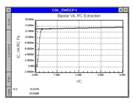
Figure 5-9: Plot of IC and VA RC Fit versus VC.
