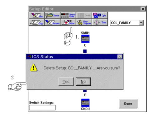
Figure 2-19: How to Delete a Test Setup.
