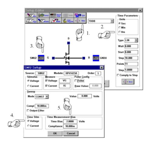
**Figure 2-12:** Configuring Source Units for Win4145 Time Measurements.
