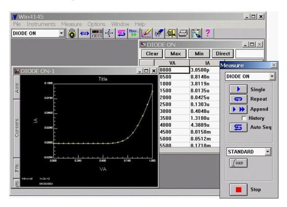
**Figure 1-11:** A Plot Window is Dynamically Linked to the Corresponding Data Window Spreadsheet.
