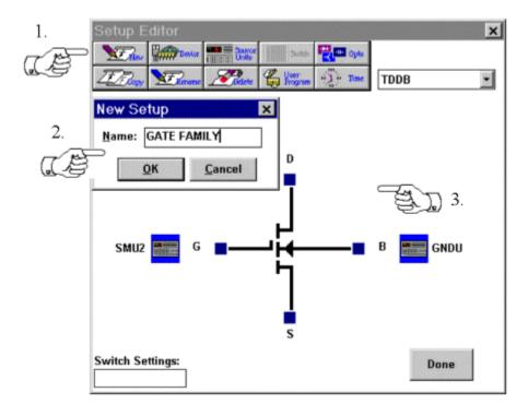
Figure 2-15: How to Create a New Test Setup.
