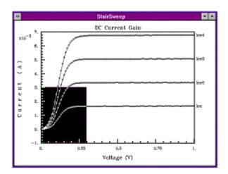
After clicking on the tool bar ZOOM button, move the Zoom Cursor to a position on the plot window that will be the corner reference of the new plot. Click and drag the mouse in order to designate the boundaries of the zoomed view.
