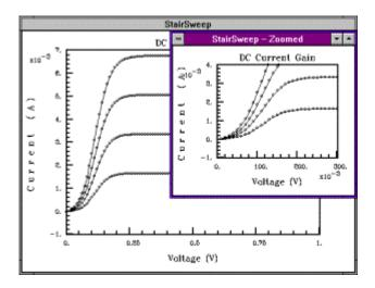
The updated plot window will be displayed after the mouse button is released. In this view, the updated plot window is an enlargement of the 4mA by 0.3V area of the original plot window.
