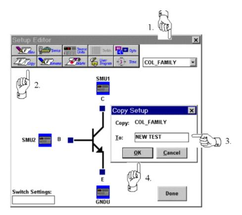
Figure 2-20: How to Copy a Test Setup.
