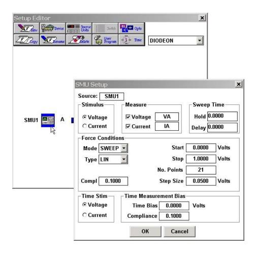
**Figure 2-10:** How to Display a Setup Dialogue Box When a Single Source Unit is Connected to the Device Schematic Pin.
