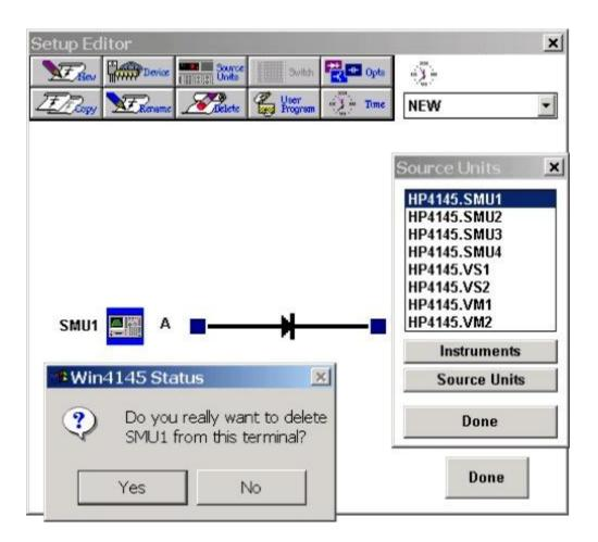
Figure 2-9: How to Remove an Instrument/DUT Connection
