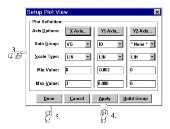
Figure 6-2: How to Create a New Plot
