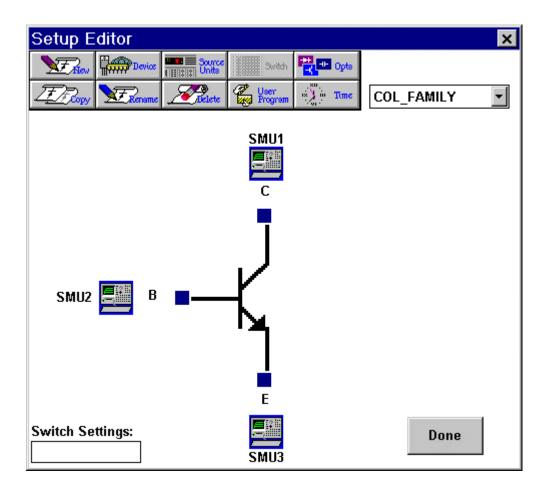
**Figure 2-4:** The Setup Editor is Used to Document Instrument/DUT Connections and Configure Instrument Setup Conditions.
