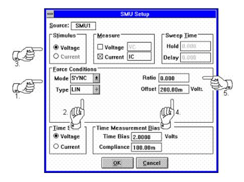
Figure 2-29: How to Source a Synchronized Sweep Signal
