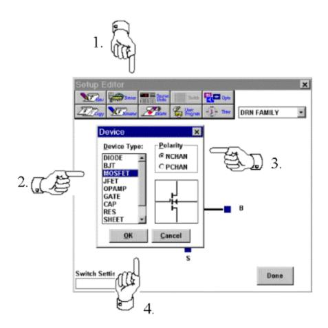
Figure 2-5: How to Select the Device Schematic.
