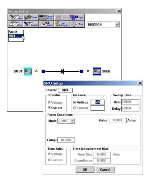
**Figure 2-11:** How to Display a Setup Dialogue Box When Multiple Source Units are Connected to the Device Schematic Pin.
