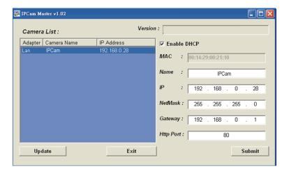
Use the supplied IPCam Master software to find the IP camera on a network and configure basic settings.
