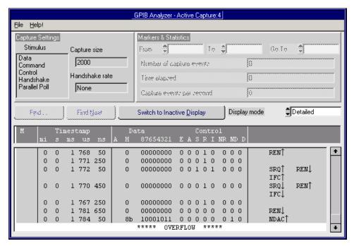
Figure 3-1. Overflow Error
