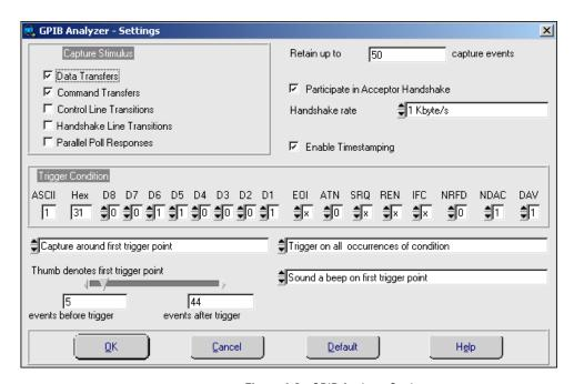
Figure 4-3. GPIB Analyzer Settings
