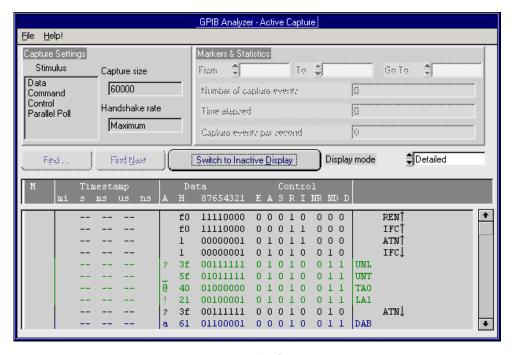
**Figure 4-2.** Capture Display Window
