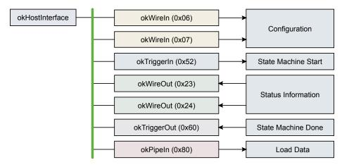
Each instance of an endpoint has an associated address (shown in parentheses) so it may be accessed independent of other endpoints. In this example, two Wire In endpoints setup the configuration for the design and two Wire Out endpoints relay status information back to the PC. The Trigger In endpoint is used to initiate a state machine and a Trigger Out endpoint is used to indicate the completion of the state machine. A Pipe In endpoint is used to load data into a memory within the design.
