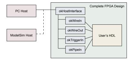
The goal of this type of simulation model is to simulate the complete FPGA design without having to make changes specific to the simulation model. In reality, many designs will require some modification, but in this case the host can be simulated as realistically as possible.
