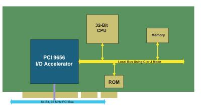
Figure 1-5. PCI 9656 PCI Adapter Card with C or J Mode Processor
