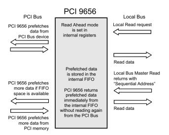
Figure 3-4. Direct Master Read Ahead Mode
