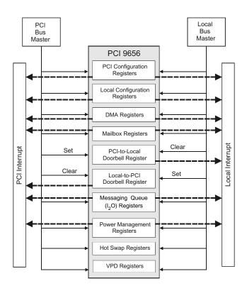
Figure 4-4. PCI 9656 Internal Register Access
