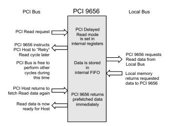
Figure 5-8. Direct Slave Delayed Read Mode
