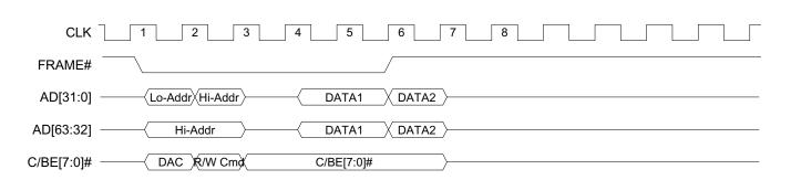
Figure 3-11. PCI Dual Address Cycle Timing
