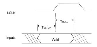
Figure 13-1. PCI 9656 Local Input Setup and Hold Timing
