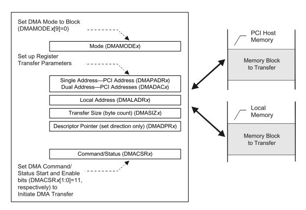
Figure 3-12. DMA Block Mode Initialization (Single Address or Dual Address PCI)
