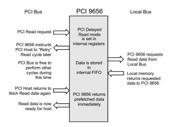
Figure 3-8. Direct Slave Delayed Read Mode
