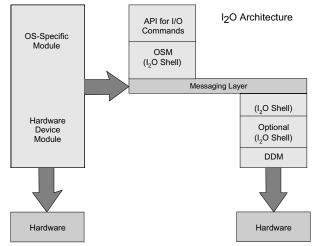
Figure 7-2. Driver Architecture Compared
