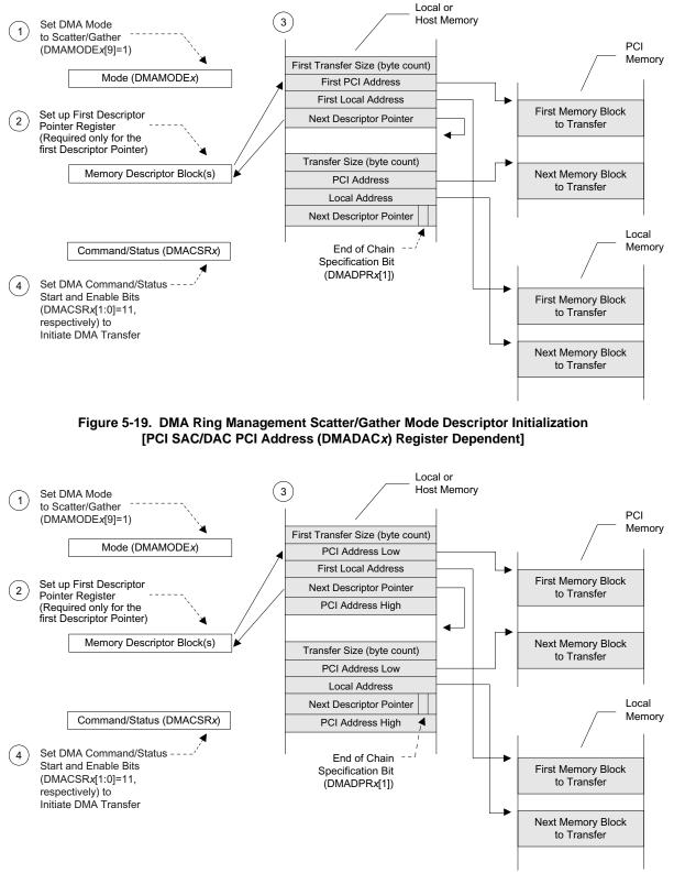
Figure 5-20. DMA Ring Management Scatter/Gather Mode Descriptor Initialization [DAC PCI Address (DMAMODEx[18]) Descriptor Dependent (PCI Address High Added)]
