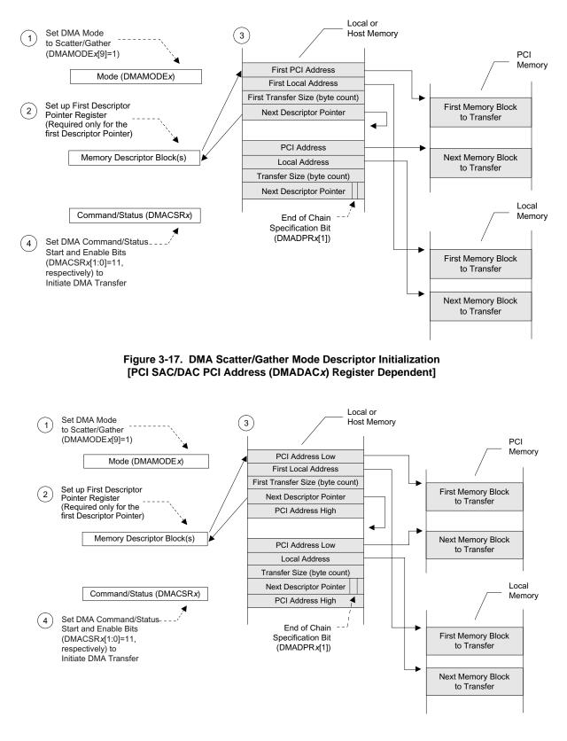
Figure 3-18. DMA Scatter/Gather Mode Descriptor Initialization [DAC PCI Address (DMAMODEx[18]) Descriptor Dependent (PCI Address High Added)
