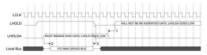
**Notes:** In response to the PCI 9656 assertion of LHOLD, the external Local Bus Arbiter asserts LHOLDA to grant the Local Bus to the PCI 9656. In Timing Diagram 4-1, the Local Bus Arbiter asserts LHOLDA immediately upon detection of LHOLD assertion; however, the Local Bus Arbiter has the option, if necessary, to assert LHOLDA significantly later.
