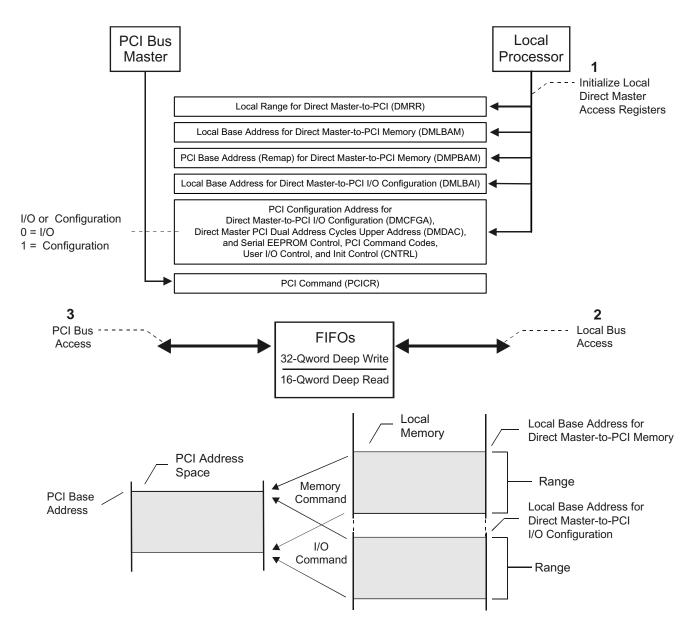
Figure 5-1. Direct Master Access of the PCI Bus
