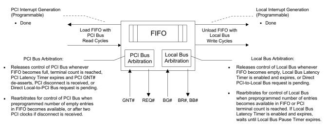
Figure 3-22. PCI-to-Local Bus DMA Data Transfer Operation
