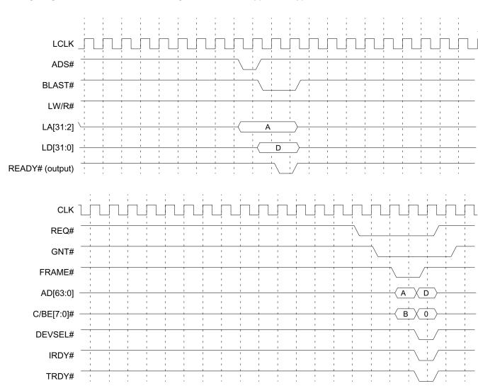
Timing Diagram 5-8. Direct Master Configuration Write – Type 0 or Type 1
