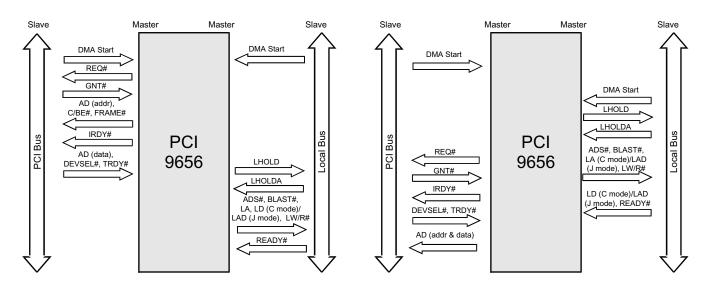
Figure 5-13. DMA, PCI-to-Local Bus
