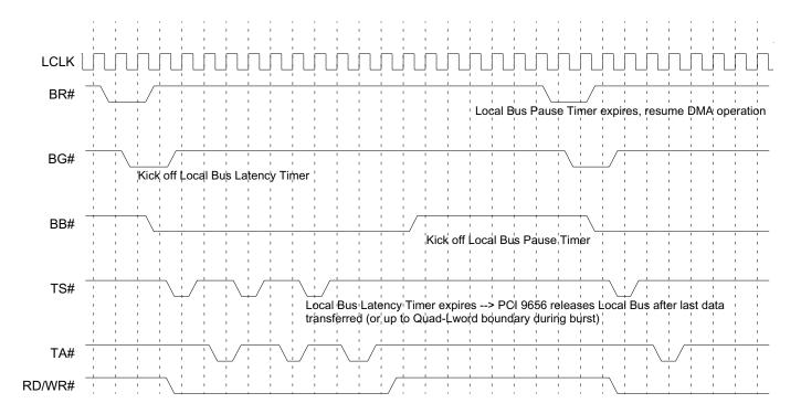
Timing Diagram 3-26. Local Bus Latency Timer (Eight Clocks) and Pause Timer (Four Clocks) in DMA Operation
