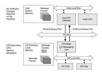
Figure 7-1. Typical I<sub>2</sub>O Server/Adapter Card Design
