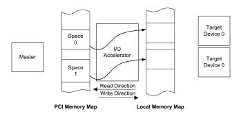
Figure 1-2. Direct Slave Address Mapping
