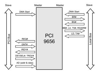
Figure 3-14. DMA, Local-to-PCI Bus
