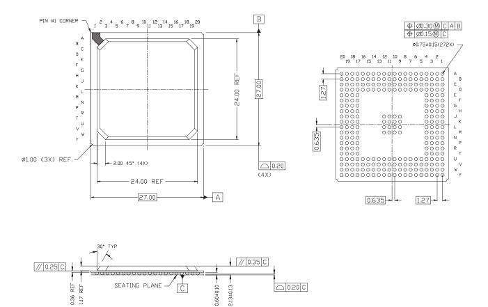
Figure 14-1. PCI 9656 Mechanical Dimensions
