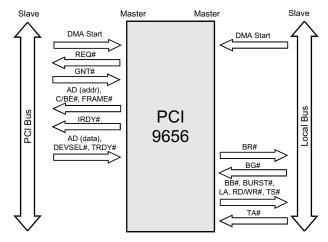
Figure 3-13. DMA, PCI-to-Local Bus
