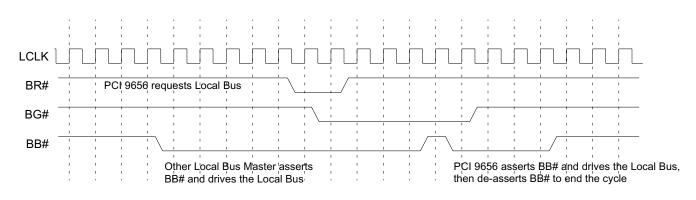
**Note:** Timing Diagram 2-1 was created using the Timing Designer tool. It is accurate and adheres to its specified protocol(s). This diagram shows transfers and signal transitions, but should not be relied upon to show exactly, on a clock-for-clock basis, where PCI 9656-driven signal transitions will occur.
