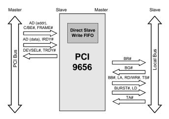
Figure 3-6. Direct Slave Write
