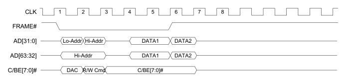
Figure 5-5. PCI Dual Address Cycle Timing
