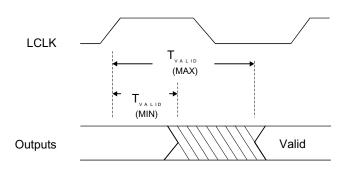
Figure 13-2. PCI 9656 Local Output Delay
