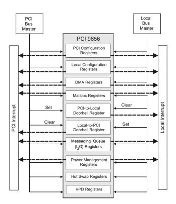
Figure 2-4. PCI 9656 Internal Register Access
