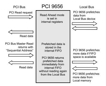
Figure 3-9. Direct Slave Read Ahead Mode
