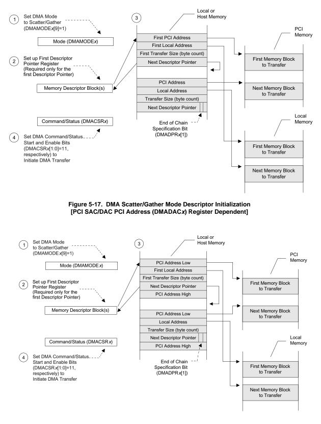
Figure 5-18. DMA Scatter/Gather Mode Descriptor Initialization [DAC PCI Address (DMAMODEx[18]) Descriptor Dependent (PCI Address High Added)]
