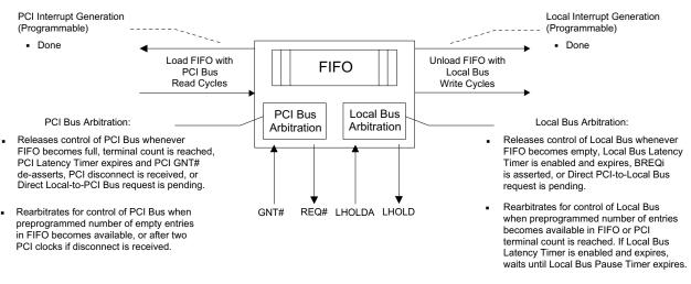
Figure 5-22. PCI-to-Local Bus DMA Data Transfer Operation
