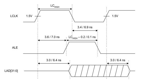
Figure 13-3. PCI 9656 ALE Output Delay to the Local Clock
