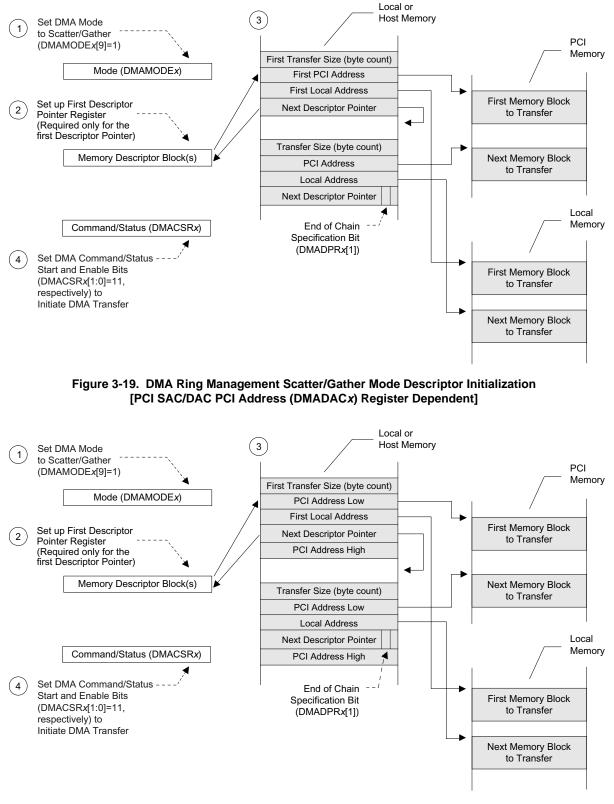
Figure 3-20. DMA Ring Management Scatter/Gather Mode Descriptor Initialization [DAC PCI Address (DMAMODEx[18]) Descriptor Dependent (PCI Address High Added)]
