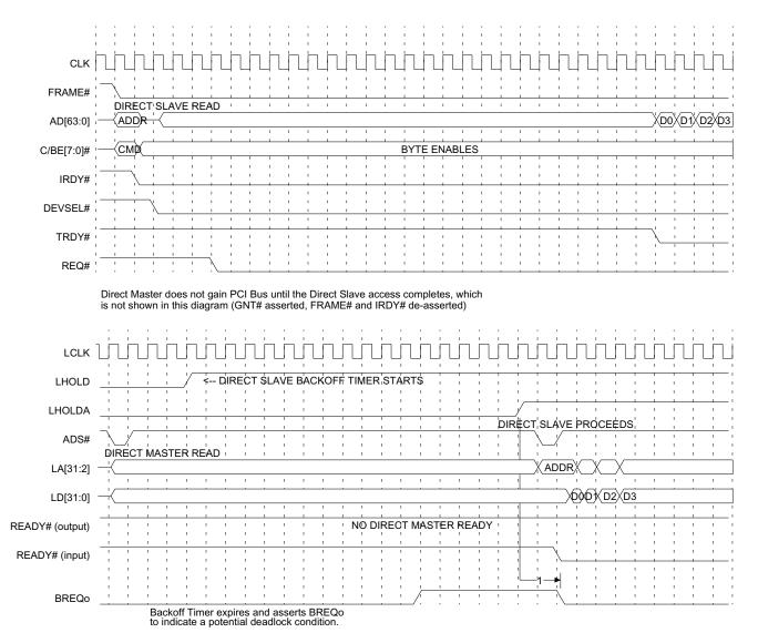
**Notes:** For partial deadlock, Direct Slave Retry Delay Clocks bits (LBRD0[31:28]) can be used to issue Retrys to the Direct Master attempting the Direct Slave access.
