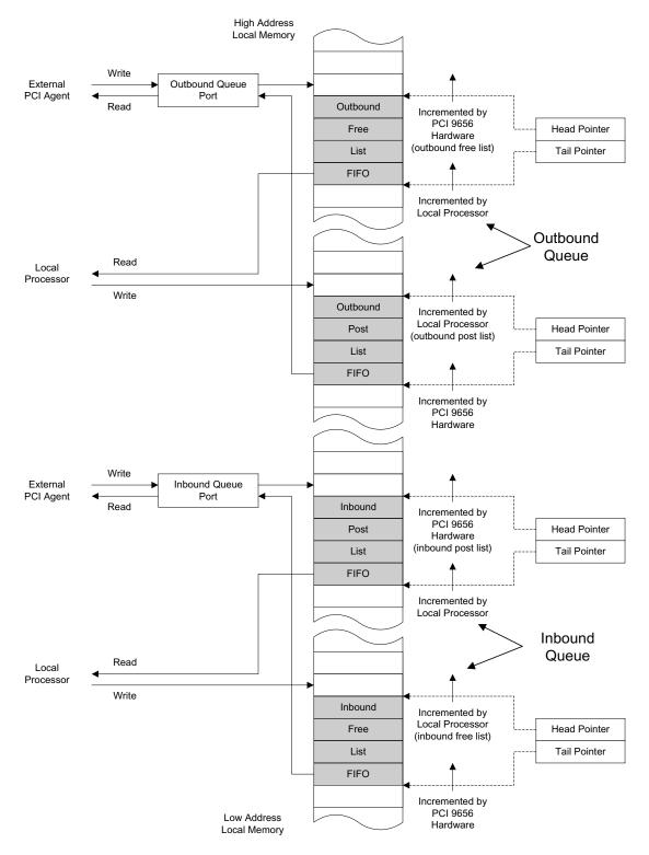
Figure 7-3. Circular FIFO Operation
