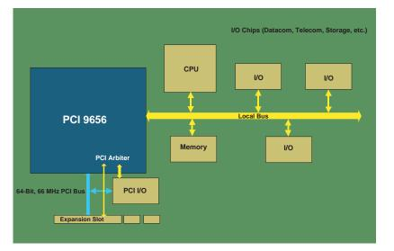
Figure 1-7. PCI 9656 Embedded Host System with Generic Host CPU
