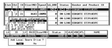
Choose "View and Edit SCSI Drives" on the main menu, press **[ENTER]**. Move the cursor bar to a SCSI drive that is not assigned to a logical drive or as a spare drive (usually indicated as a "New Drive"), and then press **[ENTER]**.
