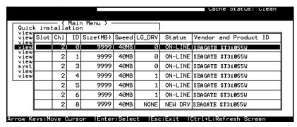
Choose "View and Edit SCSI Drives" in the main menu. All drives attached to the drive channels will be displayed on the screen.
