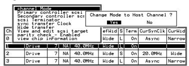
All channels can be changed into host mode or drive mode. Choose the channel you wish to change, then press **[ENTER]**. Choose "Channel Mode," then press **[ENTER]**. A dialog box will appear asking you to confirm the change.
