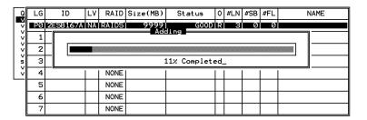
Upon completion, there will appear a confirming notification. The capacity of the added drive will appear as an unused partition.
