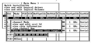
This function displays device port names (host adapter ID) detected on a host loop. Device port names will be listed here except that of the controller's I/O processor itself.
