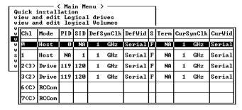
The dual loop configuration will be displayed as "channel <pair channel>." For example, channel numbers are displayed as 2<3> and 3<2> if channel 2 and channel 3 are configured in a dual loop. The data bus will be operating at the bandwidth of up to 200MB/sec.
