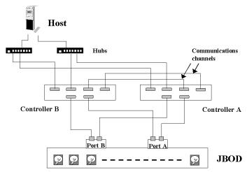
With Fibre-to-Fibre controllers, there are basically three choices with inter-communications:
