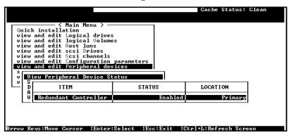
When the scanning has completed, the status will change to "Enabled."
