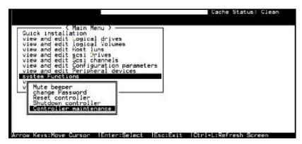
Choose "System Functions" in the main menu, then press **[ENTER].** The System Functions menu will appear. Move the cursor bar to an item, then press **[ENTER].**
