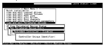
Controller Unique Identifier is **required** for operation with the **Redundant controller configuration**. The controller will automatically notify users to enter a unique identifier when the first logical drive is created in a dual-controller system.
