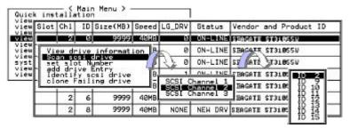
If there is a drive connected after the array is started, choose a drive and press **[ENTER].** Choose "Scan SCSI drive", then press **[ENTER].** The menu may vary according to the drive status. Choose the drive channel and SCSI ID of the drive you wish to scan, then press **[ENTER].**
