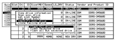
Move the cursor bar to the drive you wish to identify, then press **[ENTER].** Choose "Identify SCSI drive," then choose "flash all drives" to flash the read/write LEDs of all the drives in the drive channel. Choose **Yes**.
