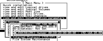
4. The controller will take a while formatting a small storage sector on each physical drive before logical drives can be successfully initialized. When the initialization process is complete, ftp RAIDWatch programs ("grm.htm" and "grm.jar") to the designated controller IP address. You may need to transfer another file, "IFT\_bundle" to the controller for OEM definitions to work.
