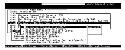
**Table 10 - 1 Peripheral Device Type Parameters**
