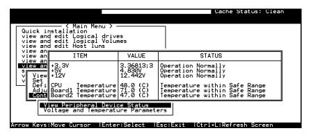
The current specimens of voltage and temperature detected by controller will be displayed on screen and will be defined as normal or out of order.
