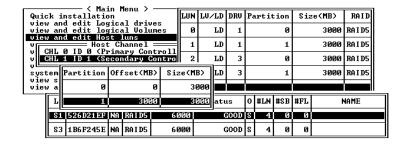
When a logical unit is selected, you may choose to "Map Host LUN" or "Create Host Filter Entry." If you select to map the logical unit directly to a host LUN without LUN masking, the particular logical unit will be accessible for all host computers connected through the network.
