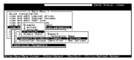
Choose "View and Edit Configuration parameters," "Controller Parameters," then press **[ENTER]**. Select "Password Validation Timeout," and press **[ENTER]**. Choose to enable a validation timeout from one minute to always check. The always check timeout will disable any configuration change without entering the correct password.
