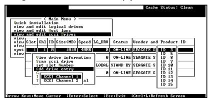
When there is an empty drive canister which currently does not contain any drive, the corresponding SCSI channel/ID will not appear in the drive information list. Assign a slot number to this empty canister and add a drive entry in order to use it later when a drive is installed.
