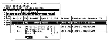
If you have primary and secondary controllers, move the cursor to the controller for the device that you wish to map; then press **[ENTER]**. You will be prompted to map a SCSI ID to a physical drive.
