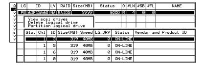
Select one of the member drives as the **"source drive"** (status indicated as ON-LINE) by pressing **[ENTER]**, a table of available SCSI drives will prompt. Select a **"new drive"** to copy the capacity of the source drive. The channel number and ID number of both the "Source Drive" and "the Destination Drive" will be indicated in the confirming box.
