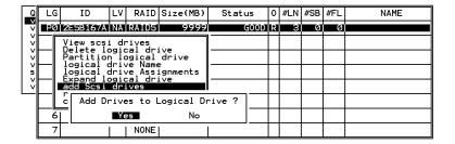
A list of available drives will appear. Select one or more drive(s) to add to the target logical drive by pressing **[ENTER].** The selected drive will be indicated by an asterisk "\*" mark.
