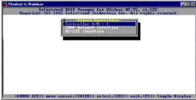
Execute the Text RAID manager program and select "Controller Maintenance." Press **[ENTER]** to proceed and then select "Upload NVRAM" as a file or "Download NVRAM" from a previously saved file.
