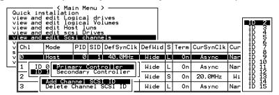
Press **[ENTER]** on one of the existing SCSI IDs. Choose "Add Channel SCSI ID," then choose to assign an ID for either the "Primary Controller" or "Secondary Controller." A list of SCSI IDs will appear. Choose a SCSI ID. **DO NOT** choose a SCSI ID used by another device on the same channel. The defaults are PID=0 and SID=1 (SCSI channel). In redundant mode, logical drives mapped to a primary ID will be managed by the primary controller, and vice versa.
