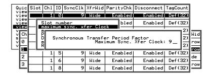
Choose "Maximum Sync. Xfer Clock," then press **[ENTER].** A dialog box will appear on the screen. Enter the clock, then press **[ENTER]**.
