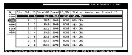
Use arrow keys to scroll down to "View and Edit SCSI Drives." This will display information of all the physical drives installed.
