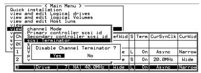
Choose the channel you wish the terminator enabled or disabled, then press **[ENTER].** Choose "SCSI Terminator", then press **[ENTER].** A dialog box will appear. Choose **Yes**, then press **[ENTER].** Terminator can also be enabled by switch jumpers, please refer to the controller hardware manual for more details.
