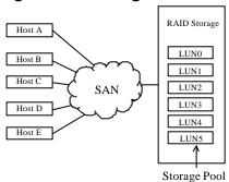
RAID-based mapping provides the centralized management for host-storage access. It is derived from the concept that storage can be divided into manageable pieces by mapping storage to different Logical Unit Numbers (LUNs). The storage can then be managed in the context of a LUN map. We then append filtering mask(s) to the LUNs making specific storage unit accessible or inaccessible to one or multiple host adapters.
