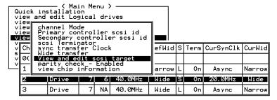
Move the cursor bar to a Drive channel, then press **[ENTER].** Select "View and Edit SCSI Target," then press **[ENTER]**.
