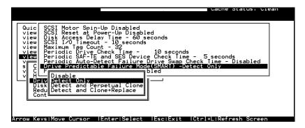
**3b.** Whenever a drive predicts symptoms of predictable drive failure, controller will issue an error message.
