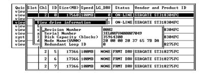
If the selected drive belongs to a drive group that is configured in a dual-loop, the "Redundant Loop ID" will be displayed here.
