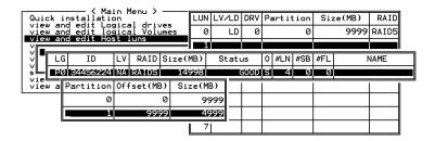
The added capacity will be included in the logical drive automatically, meaning that you do not have to perform "expand logical drive" later. However, if the logical drive has already been mapped with a host LUN, you have to map the added capacity to another host ID/LUN to make use of it. As diagrammed above, in "View and Edit Host LUN," the original capacity is 9999MB, its host LUN mapping remains unchanged and the added capacity appears as the second partition.
