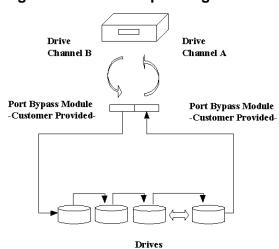
Controller firmware will automatically examine the node names and port names of all the connected drives once initiated. If devices on two different drive channels appear with the same loop ID and port name, controller will consider these two drive channels as a "dual loop."
