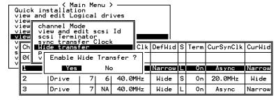
Move the cursor bar to a channel, then press **[ENTER].** Select "Wide Transfer," then press **[ENTER]**. A dialog box "Disable Wide Transfer?" or "Enable Wide Transfer?" will appear. Choose **Yes** to confirm.
