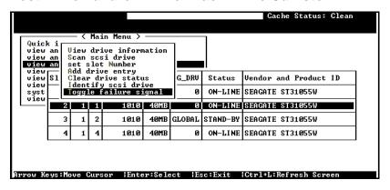
Choose the desired SCSI drive or empty drive entry from the drive information list, and press **[ENTER]**. Choose "Toggle Failure Signal" in the menu, then press **[ENTER]** to toggle the drive failure signal. The drive failure LED should light on or off followed with the toggle.
