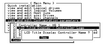
Choose "View and Edit Configuration Parameters," "Controller Parameters," then press **[ENTER]**. Choose to display the embedded controller logo or any given name on LCD. Giving a specific name to controller will help if you choose to configure a multiple number of RAID systems remotely through management software.
