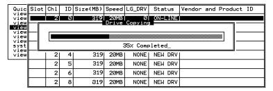
You may also quit viewing the status bar by pressing **[ESC]** to return to the previous menu screen. Select the drive indicated as "CLONING" by pressing **[ENTER]**. Select "Clone Failing Drive" again to view the progress. You may identify the source drive and choose to "View clone progress" or "Abort clone" if you happen to have selected the wrong drive.
