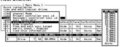
Move the cursor bar to a channel, then press **[ENTER].** Choose "Sync Transfer Clock", then press **[ENTER].** A list of the clock speed will appear. Move the cursor bar to the desired speed and press **[ENTER].** A dialog box "Change Sync Transfer Clock?" will appear. Choose **Yes** to confirm.
