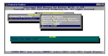
Provide location and file name, then press **[ENTER]** to proceed. The uploading or downloading process will be completed almost instantly.
