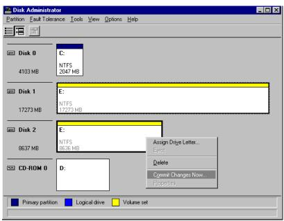
Logical Drive E: is now composed of two partitions with a total volume of 1800MB. To see this, hold down on the <Ctrl> key and select both Disk 1 and Disk2; then right-click your mouse and select "Properties."
