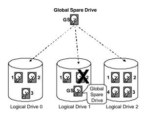
The external RAID controllers provide both Local Spare Drive and Global Spare Drive functions. On certain occasions, applying these two functions together will better fit various needs. Take note though that the Local Spare Drive always has higher priority than the Global Spare Drive.
