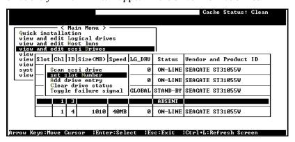
Move the cursor bar on the empty drive entry and press **[ENTER]**. Choose "Set Slot Number" in the menu, then press **[ENTER]**. Enter the slot number of this empty canister so as to use it later when a drive is installed.
