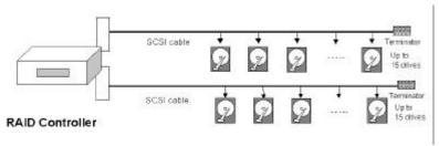
The physical connection of a RAID controller should be similar to the one shown above. Install the controller into an enclosure canister, then connect drives to the controller's SCSI/Fibre channels.
