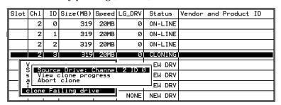
Select "clone Failing drive" again to view the current status. You may identify the source drive and choose to "view clone progress," or "abort clone" if you happen to have selected the wrong drive.
