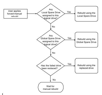
f neither Local Spare nor Global Spare is available, the controller will examine the SCSI channel and ID of the failed drive. Once the failed drive has been replaced by a healthy one, it starts to rebuild using the new drive. If there is no available drive for rebuilding, the controller will not attempt to rebuild until the user applies another forced-manual rebuild.
