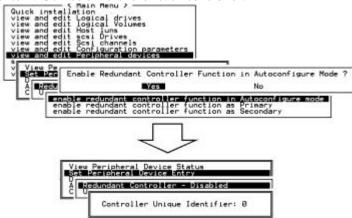
The unique identifier can also be accessed from "View and Edit Configuration Parameters"  $\rightarrow$  "Controller Parameters"  $\rightarrow$  "Controller Unique ID."
