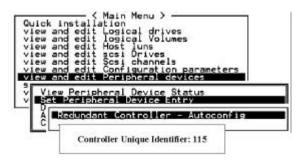
A "Controller Unique Identifier" box will appear. Enter any value from 1 to 65535, then press **[ENTER]** to proceed. The value you enter for controller unique ID should be different for each controller.
