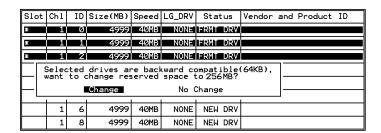
You will be prompted with the similar options using the Quick Install function. The selection box will not appear when all drives are new or that reserved space has been removed from drives.
