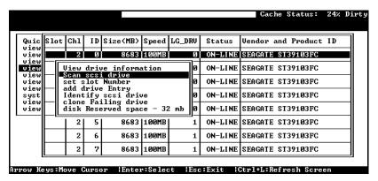
Choose "View and Edit SCSI Drives" on the main menu and use the arrow keys to move the cursor bar through connected drives. Press **[ENTER]** to choose a drive, or **[ESC]** to return to the previous menu/screen.
