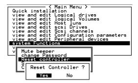
To reset the controller without powering off the system, move the cursor bar to "Reset Controller," then press **[ENTER]**. Choose **Yes** in the dialog box that follows, then press **[ENTER]**. The controller will now reset as well as power-off or re-power-on.
