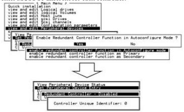
The unique identifier can also be accessed from "View and Edit Configuration Parameters"→ "Controller Parameters"→ "Controller Unique ID."
