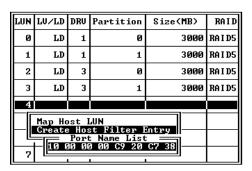
Pressing **[ENTER]** on "Add from current device list" will bring forth a list of port names detected on host loops. If you have a name list preconfigured, port names will appear with its nick names. Select a port name by pressing **[ENTER]**.
