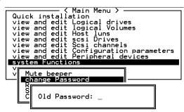
Use the controller's password to protect the array from unauthorized entry. Once the controller's password has been set, regardless of whether the front panel, the RS-232C terminal interface or RAIDWatch Manager is used, the user can only configure and monitor the RAID controller by providing the correct password.
