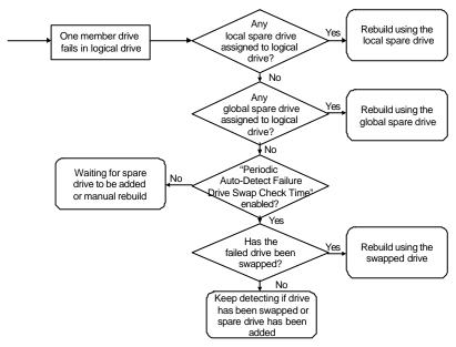
**Rebuild with Spare:** When a member drive in a logical drive fails, the controller will first examine whether there is a Local Spare Drive assigned to this logical drive. If yes, it will automatically start to rebuild.
