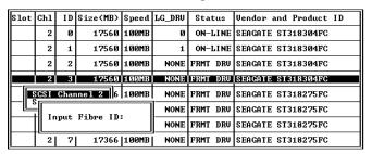
A drive enclosure usually has drive slots pre-assigned with IDs. There are occasions when an ID needs to be assigned manually to a device other than an ID provided otherwise. The "set slot number" and the "add drive entry" functions are reserved for Infortrend's Faultbus operation.
