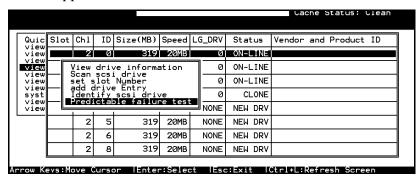
**6.** Choose "Predictable Failure Test," the controller will force the drive to simulate the predictable drive error.
