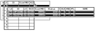
Select one or more logical drive(s) available on the list. The same as creating a logical drive, the logical drive(s) can be tagged for inclusion by positioning the cursor bar on the desired drive and then press **[ENTER]** to select. An asterisk (\*) will appear on the selected drive. Press **[ENTER]** again will deselect a logical drive.
