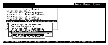
Select "View and edit Configuration parameters" on the main menu and press **[ENTER].** Choose "Disk Array Parameters," then press **[ENTER]** again. The Disk Array Parameters menu will appear.
