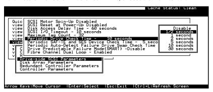
**2.** In \View and Edit Configuration Parameters\Drive-side SCSI Parameters\Drive Predictable Failure Mode <SMART>, choose one from "Detect Only," "Detect, Perpetual Clone" and "Detect, Clone+Replace."
