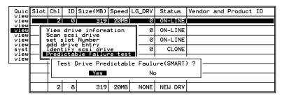
**7.** Press **[ENTER]**, and after a while (the next time the controller performs "Periodic Drive Check"), the controller will detect the error simulated by the drive. An error message will be displayed: "[1142] SMART-CH:? ID:? Predictable Failure Detected (TEST)." If this error message appears, it means the selected drive supports S.M.A.R.T. feature. If this error message does not appear, it means that this drive does not support S.M.A.R.T..
