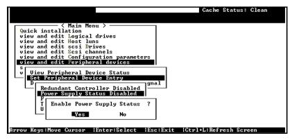
Each item of the error signal input can be individually enabled or disabled. Choose "View and Edit Peripheral Devices" in the Main Menu, then press **[ENTER]**. Select "Set Peripheral Device Entry," then press **[ENTER]**. Move the cursor to the desired item to enable or disable, and press **[ENTER]**. Choose "Yes" in the following dialog box, then press **[ENTER]** to set.
