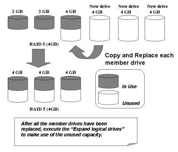
Select from main menu "View and Edit Logical Drives." Select a target logical drive, press **[ENTER]** and scroll down to choose "copy and replace drive." Press **[ENTER]** to proceed.
