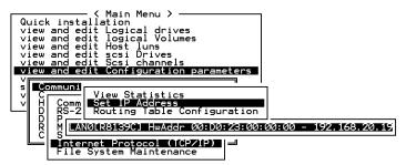
• Enter the IP address, NetMask, and Gateway values accordingly.
