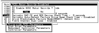
The SCSI "spin-up" decides how the SCSI drives in a Disk Array are started. When the power supply is unable to provide sufficient current for all the hard drives and controllers that are powered-up at the same time, spinning-up the hard drives serially is one of the best ways of consuming lower power-up current.
