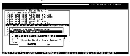
Choose "Caching Parameters", then press **[ENTER].** Select "Write-Back Cache," then press **[ENTER].** "Enabled" or "Disabled" will display the current setting with the Write-Back caching. Choose **Yes** in the dialog box that follows to confirm the setting.
