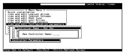
Choose "View and Edit Configuration Parameters," "Controller Parameters," then press **[ENTER]**. The current controller name will be displayed. Press **[ENTER]**. Enter the new controller name in the dialog box that follows, then press **[ENTER]**.
