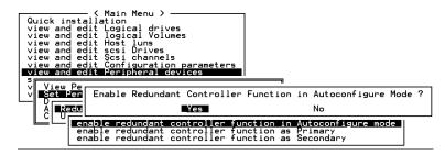
Use the arrow keys to scroll through the available options ("Primary," "Secondary," or "Autoconfigure"), then press **[ENTER]** to select "**Autoconfigure**." When prompted by "enable redundant controller function in Autoconfigure mode?," choose **Yes.**
