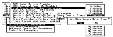
Choose "Disk Access Delay Time," then press **[ENTER]**. A list of selections will appear. Move the cursor bar on a selection, then press **[ENTER]**. Choose **Yes** in the dialog box that follows to confirm the setting.
