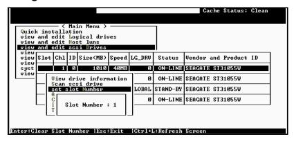
Choose "View and Edit SCSI Drives" in the Main Menu, then press [ENTER]. A list of the connected SCSI drives will appear. The "Slot" column indicates the current slot number of each SCSI drive.
