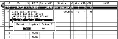
Choose the logical drive that has a failed member drive, then press **[ENTER].** Choose "Rebuild logical drive", then press **[ENTER].** When prompted to "Rebuild Logical Drive?," select **Yes**.
