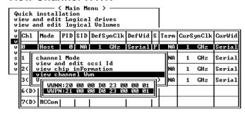
Port name is the unique eight-byte address assigned to a FC port.
