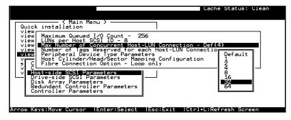
From the main menu, select "View and Edit Configuration Parameters," "Host-side SCSI Parameters," then press **[ENTER]**. Choose "Max Number of Concurrent Host-LUN Connection," then press **[ENTER]**. A list of available selections will appear. Move the
