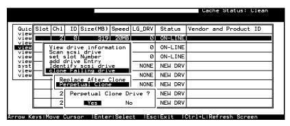
The controller will automatically start the cloning process by using the existing "stand-by" (local/global spare drive) to clone the source drive (the target member drive with predicted error).
