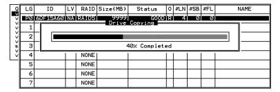
Completion of the Copy and Replace process will be indicated by a notification message. Follow the same method to copy and replace every member drive with drives of higher capacity. You may now perform "Expand Logical Drive" to make use of the capacity brought by the new drives and then map the additional capacity to a Host LUN.
