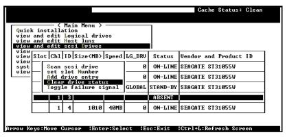
Before an empty drive entry can be removed, the slot number has to be deleted first. Please refer to the above paragraph on how to delete the slot number.
