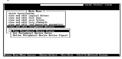
Choose "View and Edit Peripheral Devices" in the Main Menu and press **[ENTER]**. Select "View Peripheral Device Status" in the menu and press **[ENTER]**.
