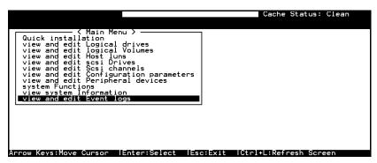
The controller can store up to 1000 event logs for use in modifying the configuration.
