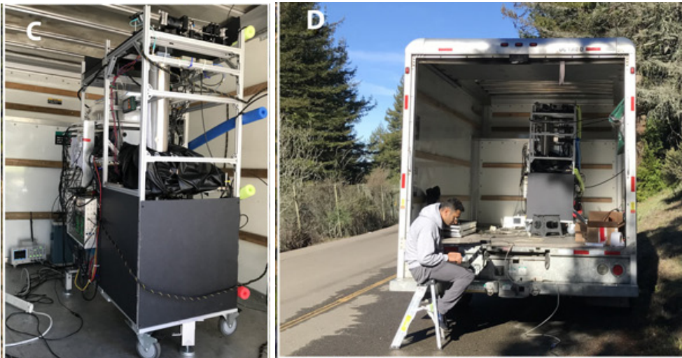
Mobile atomic gravimeter from Mueller lab (UC Berkeley)
