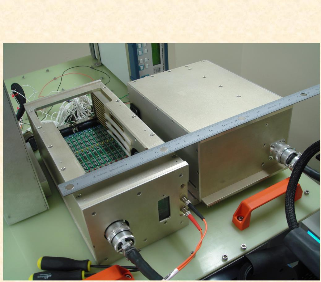
Figure 3: Detector control electronics built by Astronomical Research Cameras, Inc. The SIDECAR has the same capability as this set of electronics.
