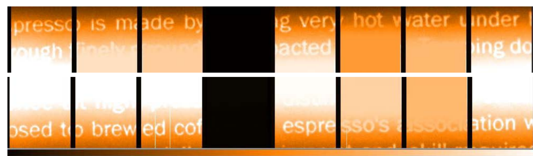
Figure 3: (Left) Lab Test set-up with NGC DFE & PS; (Right) Warm first light images showing projection on 8 channels each (top and bottom). Two outputs of this very early sample are non-functional.
