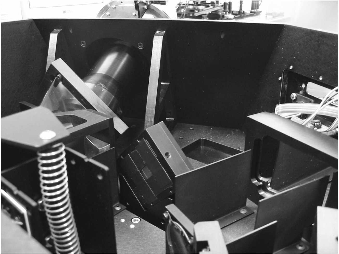
Figure 5. The interior of RITMOS, as viewed from the top front corner on the imaging side. The diamond-shaped structure at the center houses the DMD, which is the lighter area within the structure. The DMD is rotated so that the mirror diagonals are perpendicular to the primary optical plane. In the left foreground is the calibration lamp assembly; behind that, from front to back, are the collimator, the grating, and the re-imager lens barrel. The grating, like the DMD, is rotated by 45^\circ . Both the grating and the lens barrel are tilted up from the primary optical plane. The spectroscopy CCD is visible above the back wall, behind the lens barrel. The Offner relay is to the right of the DMD.
