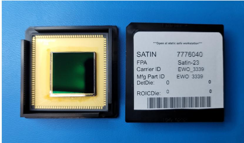
Figure 1. The image shows the VIRGO-V23 detector on the left and the container lid on the right.
