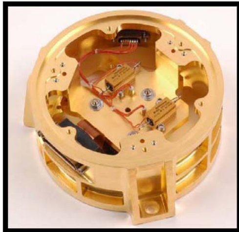
FPA - Backside - Cover Removed
