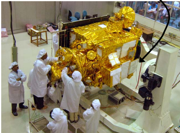
Completion of Chandrayaan-1 spacecraft integration Moon Mineralogy Mapper is white square at end of arrow
