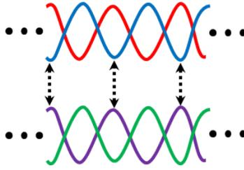
Figure 18: Two neighboring twisted pairs of the same twist rate.
