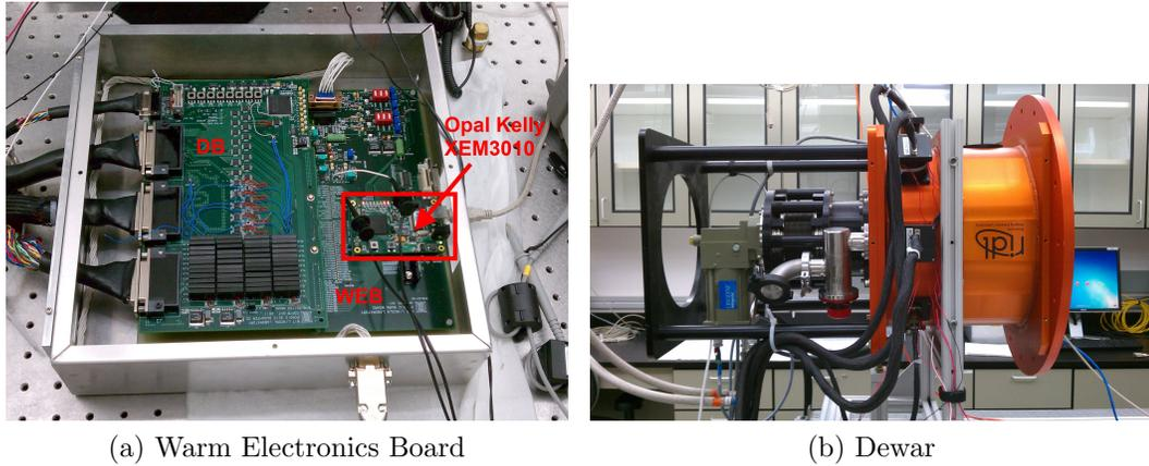
Figure 2: (a) The interconnected WEB and DB; (b) the dewar, a cryogenic test chamber for the detectors.
