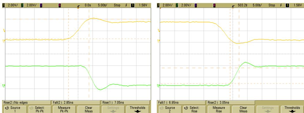
Figure 32: Oscilloscope capture demonstrating the effects of a Schmitt-trigger on edge times. Channel 1 (yellow) is the input, and channel 2 (green) is the output.
