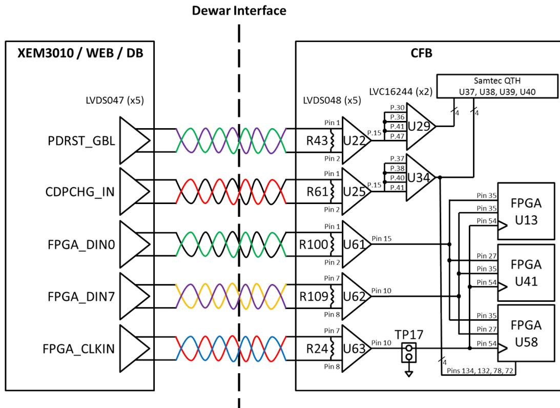
Figure 15: Imaging system signal path diagram for signal integrity analysis.
