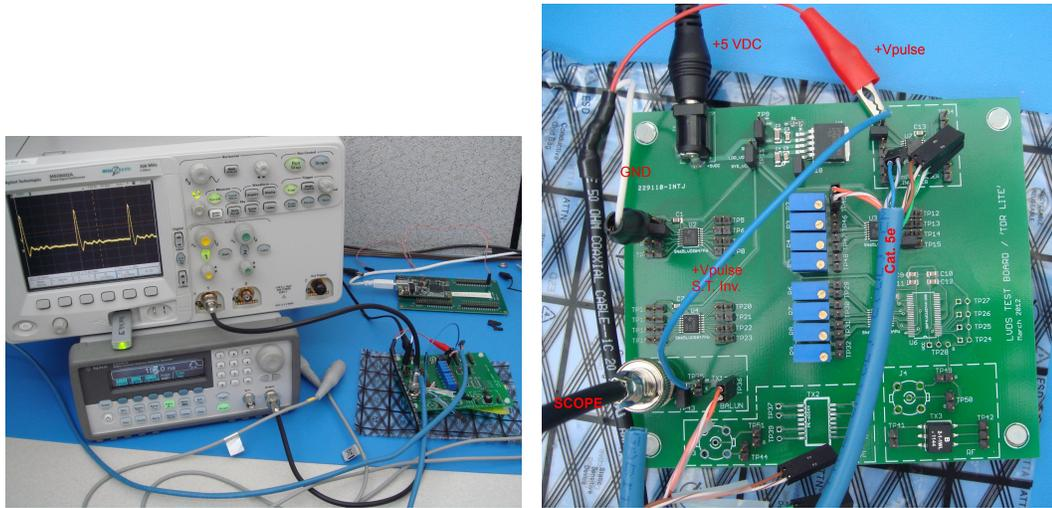
Figure 34: Bench setup of balun TDR.
