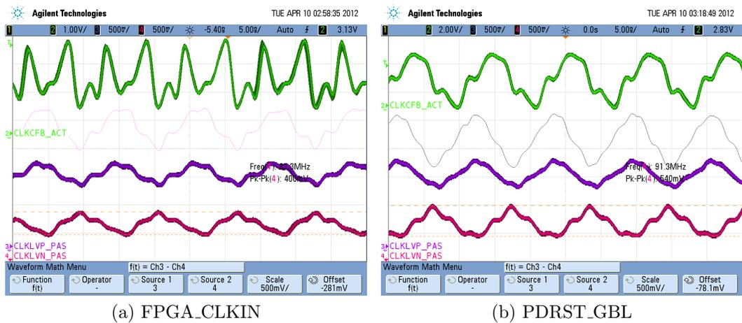
Figure 41: Comparison of a 90 MHz signal over the FPGA\_CLKIN and PDRST\_GBL signal paths terminated on the CFB. Channel 2 (green) is the active probe at the LVDS receiver output. Channel 3 (purple) and channel 4 (pink) show the inputs to the LVDS receiver. The math function shows the difference between channels 3 and 4.
