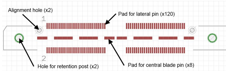
Figure 4: PCB footprint for the Samtec QTH high-speed mezzanine connectors. These connectors feature pins with 0.5 mm pitch, and retention posts for secure mating with the Samtec QSH connectors on the detectors.
