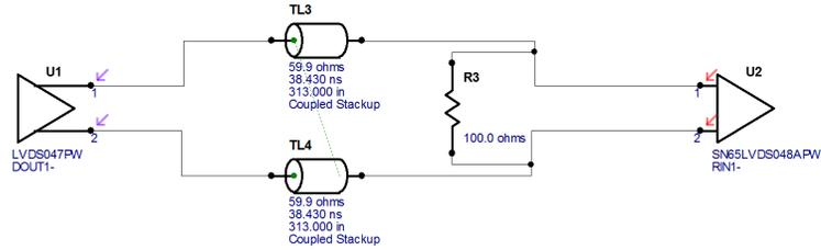
(a) LineSim free-form schematic of cat. 5e cable
