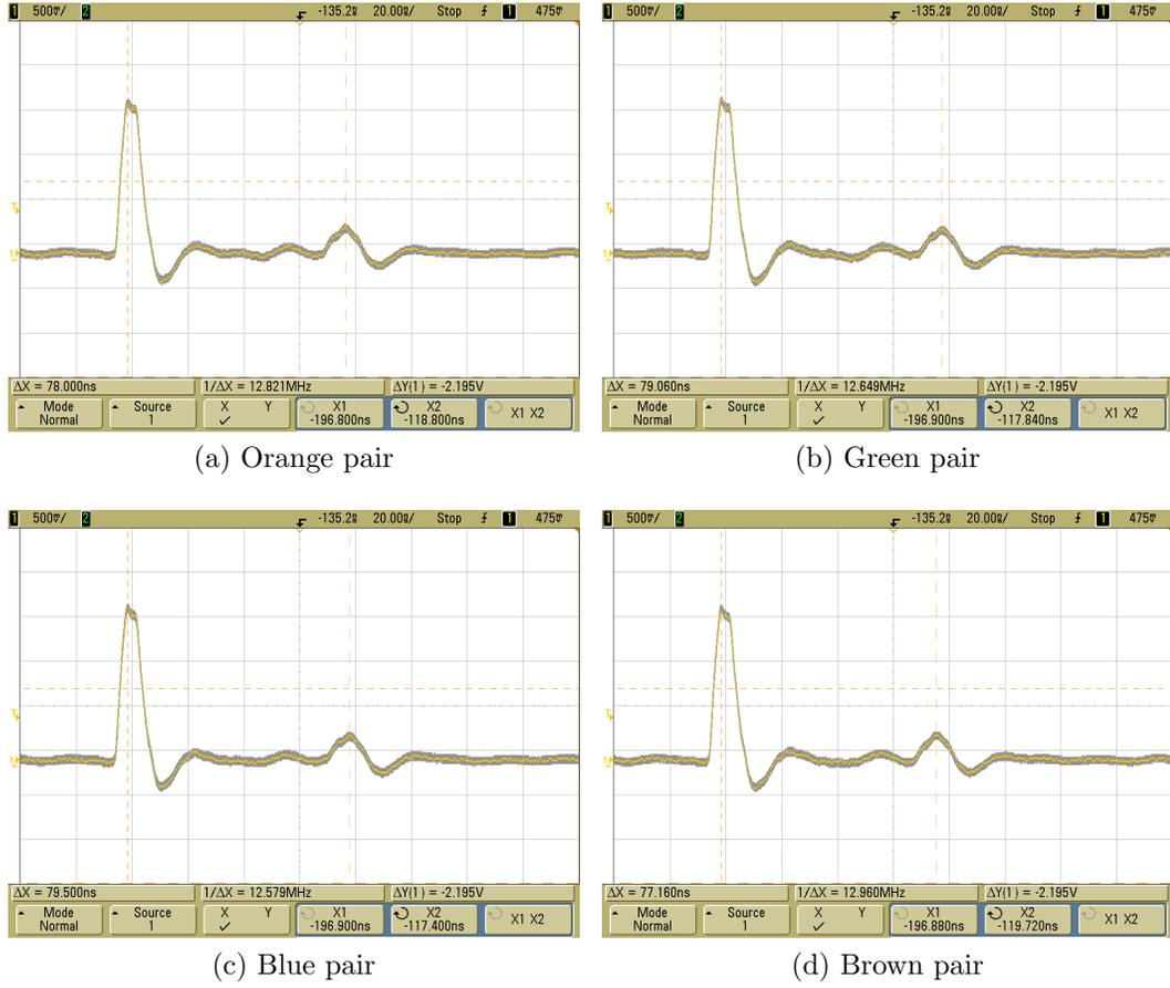
Figure 36: Round-Trip Time measurement of cat. 5e using TDR.
