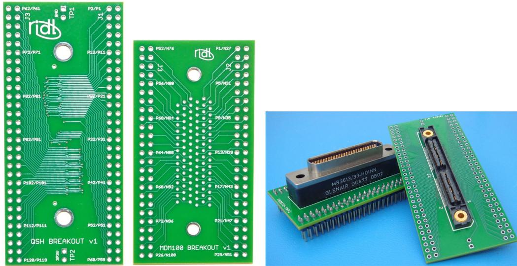
Figure 7: Custom breakout boards designed for the Samtec QSH and M83513 100-position microminiature connectors.
