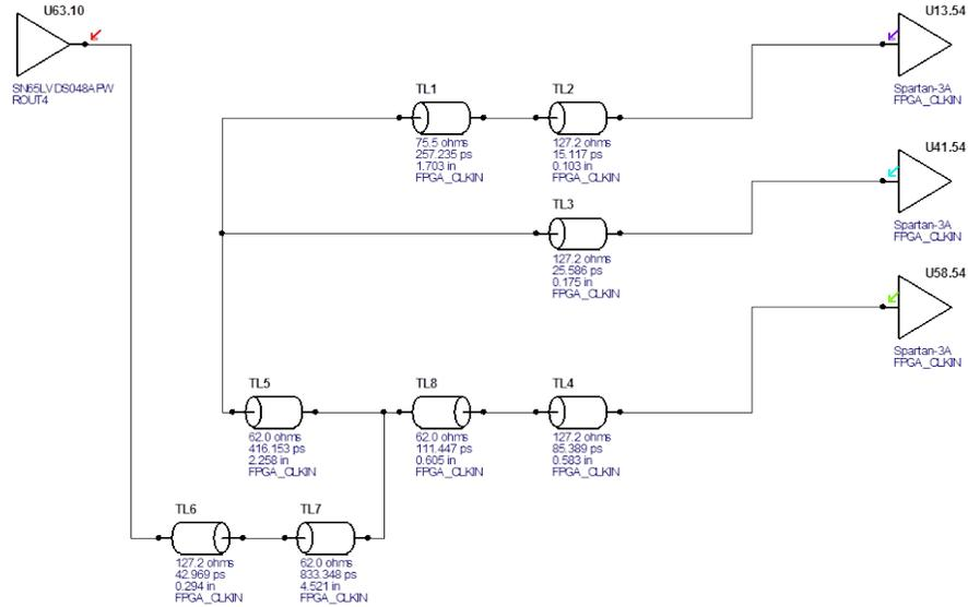
Figure 43: HyperLynx LineSim free-form schematic of FPGA\_CLKIN.
