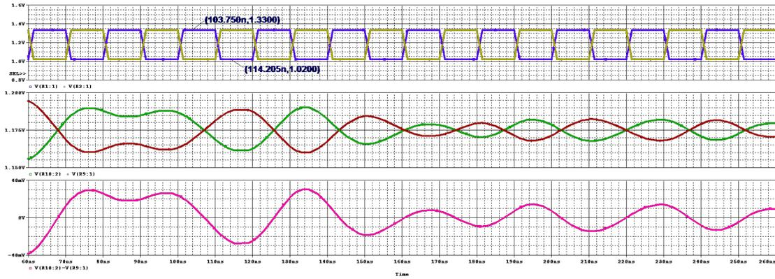
Figure 22: PSPICE simulation of the RLCG twisted pair model at 50 MHz.
