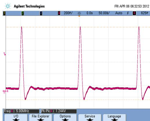
Figure 37: Balun TDR of FPGA\_CLKIN terminated at R24 on the CFB.
