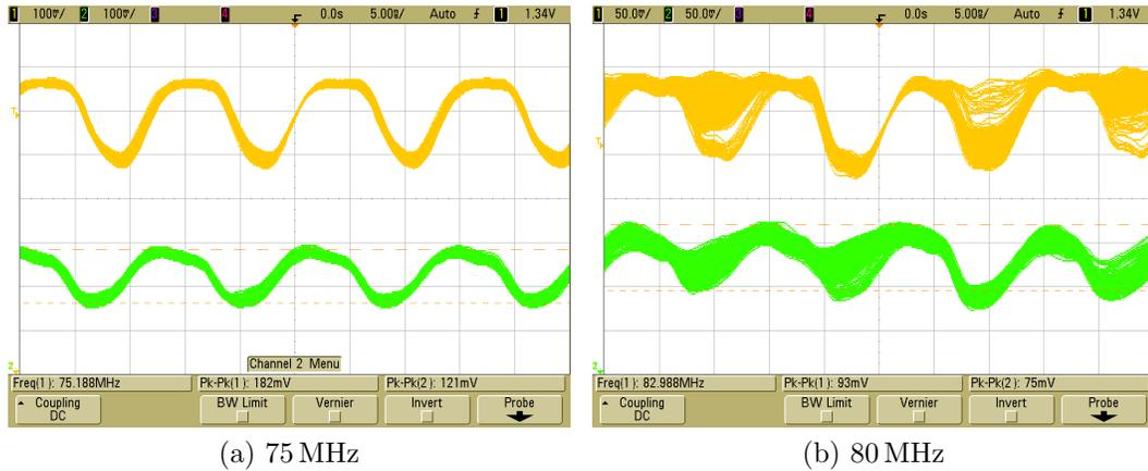
Figure 19: Oscilloscope captures across the system cabling. The yellow trace (channel 1) is probing the positive output of the LVDS driver on the DB. The green trace (channel 2) is probing the positive input of the LVDS receiver on the CFB.
