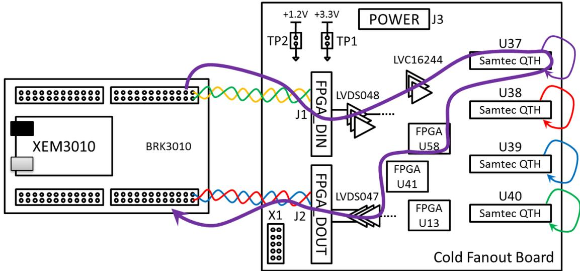
Figure 8: Cold Fanout Board loop-back test setup. The thick purple arrow is an example signal path. Note that the loop-back test verifies the functionality of each component on the CFB. This general setup was also used during BER testing.
