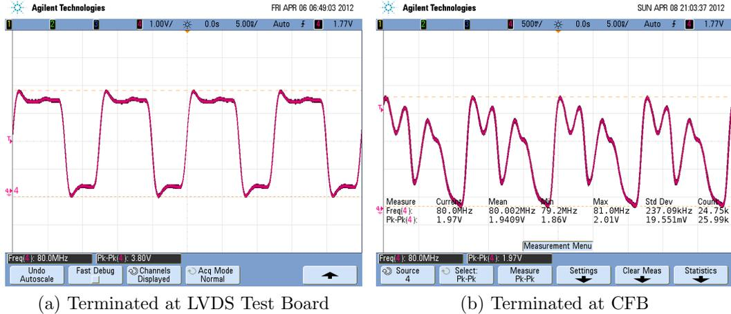
Figure 39: The output of the LVDS receiver when the input (FPGA\_CLKIN) is terminated on (a) the LVDS/TDR Test Board with  $R_{\text{term}} = 100.23\ \Omega$ ; and (b) the CFB with  $R_{\text{term}} = 100.14\ \Omega$ .
