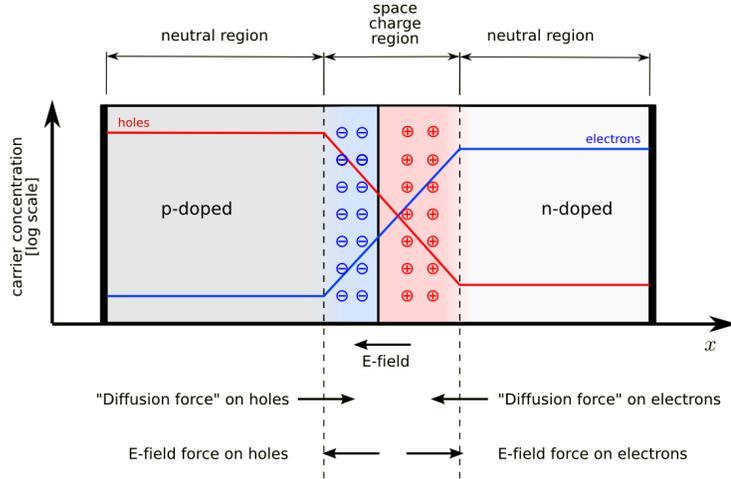
Figure 3: PN junction in thermal equilibrium and zero bias voltage [2].
