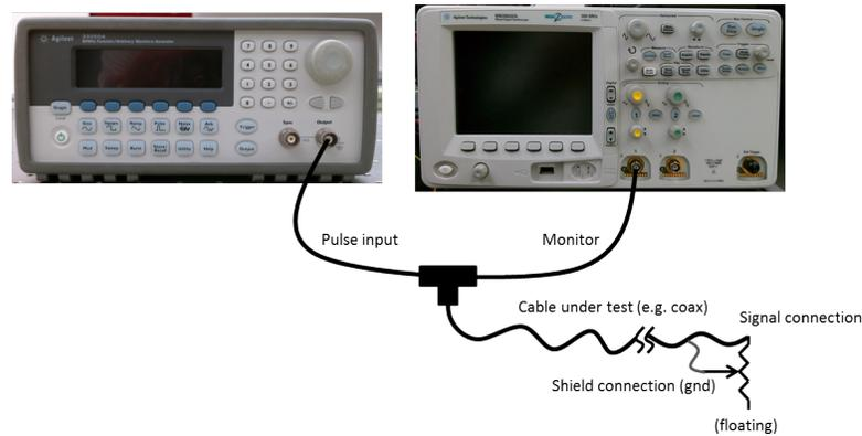
Figure 31: A single-ended TDR constructed with common lab equipment.
