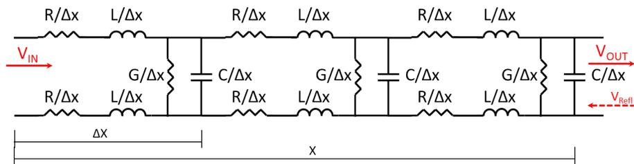
Figure 20: Balanced three-segment RLCG transmission line model.
