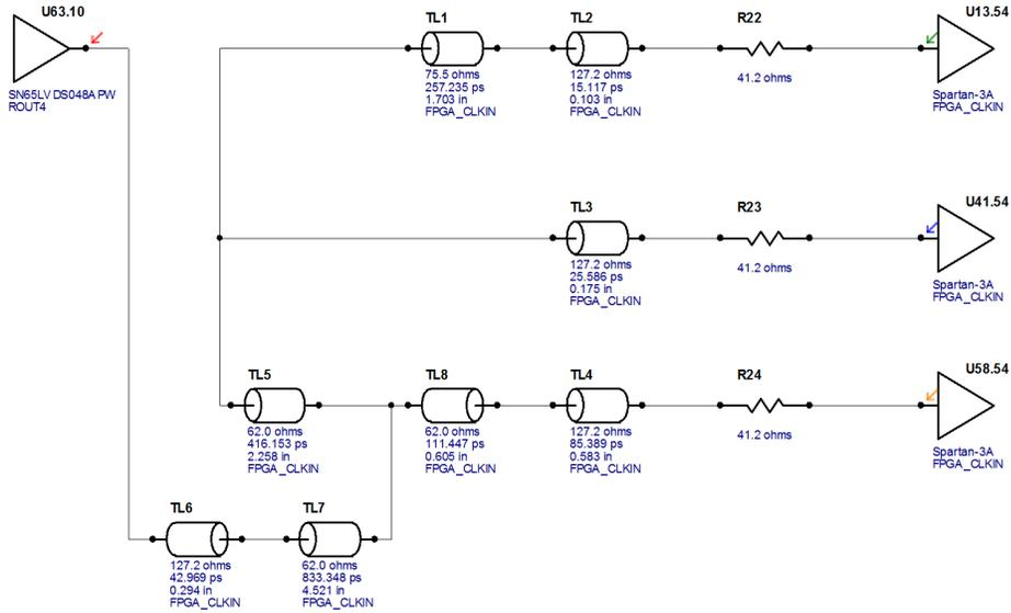
Figure 54: HyperLynx LineSim free-form schematic of FPGA\_CLKIN with series end termination. The termination values shown were calculated with the HyperLynx termination wizard.
