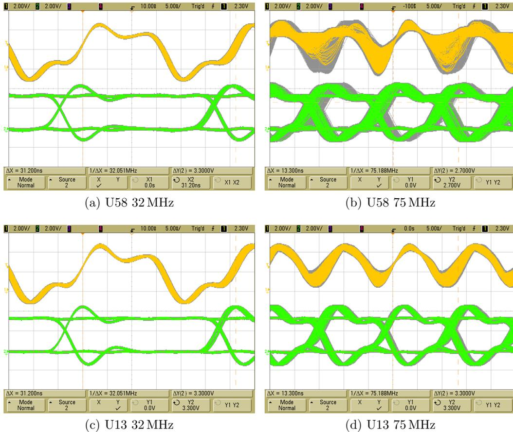
Figure 17: A sampling of eye diagrams using the full system. Channel 1 (yellow) is the FPGA\_CLKIN clock signal, and channel 2 (green) is the eye diagram formed by the pseudorandom sequence. The U58 FPGA was considered worst case and the U13 FPGA was considered best case. Both reside on the Cold Fanout Board.
