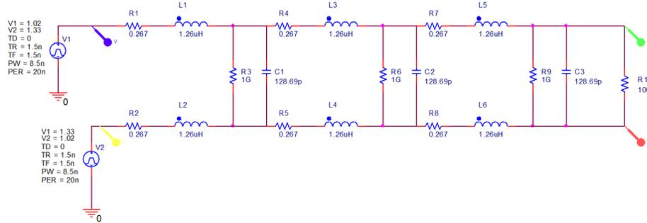
Figure 27: OrCAD schematic of RLCG model using category 5e cable parameters.
