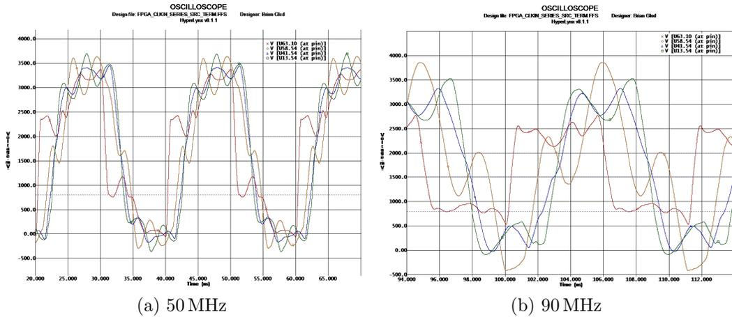
Figure 51: LineSim simulation of the FPGA\_CLKIN net at 50 MHz and 90 MHz using series source termination. The red trace is at the output of the LVDS receiver (U63, pin 10). The orange trace is at FPGA U58 pin 54, blue is at FPGA U41 pin 54, and green is at FPGA U13 pin 54.
