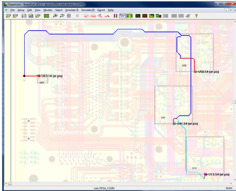
Figure 42: Section of the Cold Fanout Board layout imported into HyperLynx BoardSim. The highlighted net is FPGA.CLKIN, which carries the shared clock signal for the three cold FPGAs. Device U63.10 is the output of the LVDS receiver; devices U13.54, U41.54, and U58.54 are the FPGA clock input pins.
