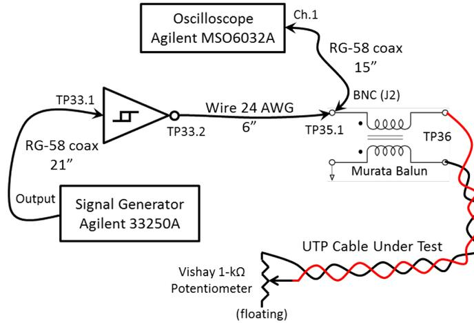
Figure 33: Balun TDR connection diagram.
