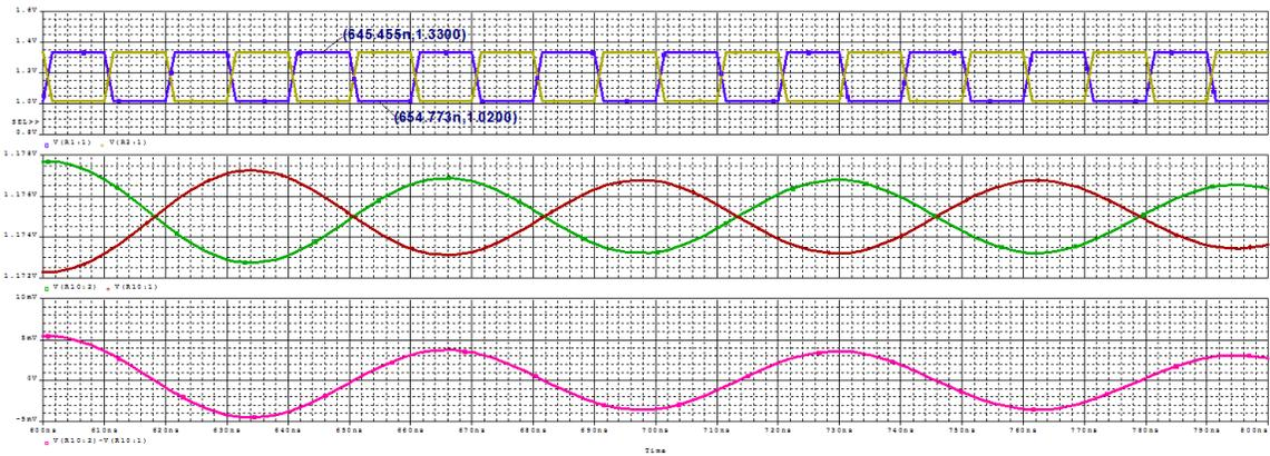
Figure 28: PSPICE simulation of the RLCG category 5e model at 50 MHz.
