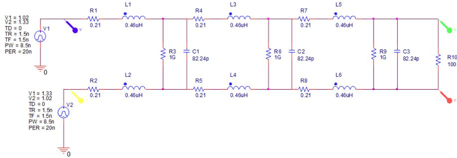
Figure 21: OrCAD schematic of RLCG model using system parameters.
