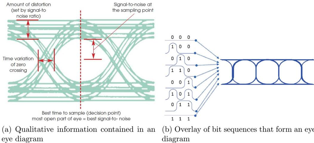
Figure 16: (a) Shows the qualitative information contained in an eye diagram. The most important are the vertical eye opening (noise) and the width of the crossing point (jitter) [10]. (b) Shows an overlay of the bit sequences that form an eye diagram [11].
