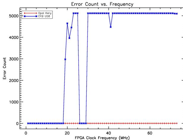
Figure 10: BER test results with the full system setup using the binary counter pattern from 1 MHz to 73 MHz with 1 MHz steps and 5 iterations at each step.
