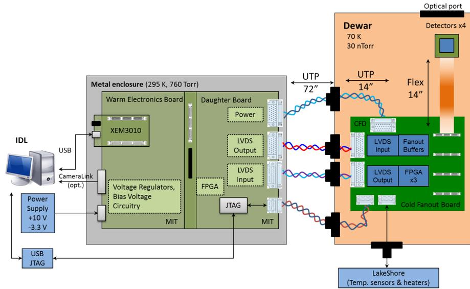
Figure 1: Diagram of the full system.
