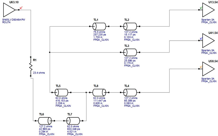
Figure 50: HyperLynx LineSim free-form schematic of FPGA.CLKIN with series source termination.
