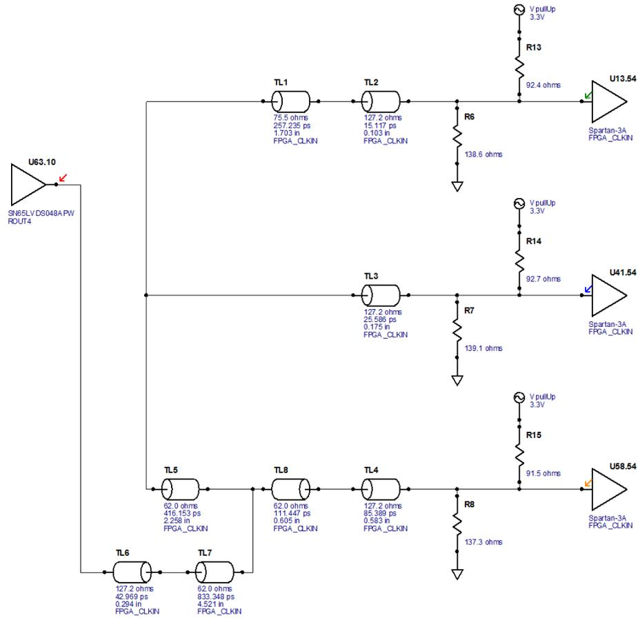
Figure 52: HyperLynx LineSim free-form schematic of FPGA\_CLKIN with split end termination. The termination values shown were calculated with the HyperLynx termination wizard.
