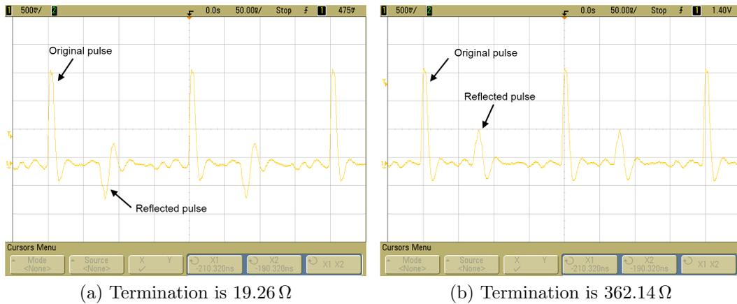
Figure 35: Effects of mismatched termination on cat. 5e cable. The optimal termination for cat. 5e is 100  $\Omega$ .
