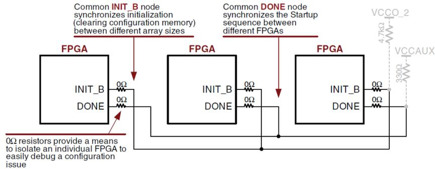
Figure 6: Xilinx User Guide 332 recommended DONE and INIT\_B pin configuration for daisy-chained or broadside JTAG configurations [4]. The CFB was designed in a similar manner, but used 1.0 k $\Omega$  pull-up resistors on the ganged DONE and INIT\_B outputs instead of 330  $\Omega$  and 4.7 k $\Omega$  as shown in the figure.
