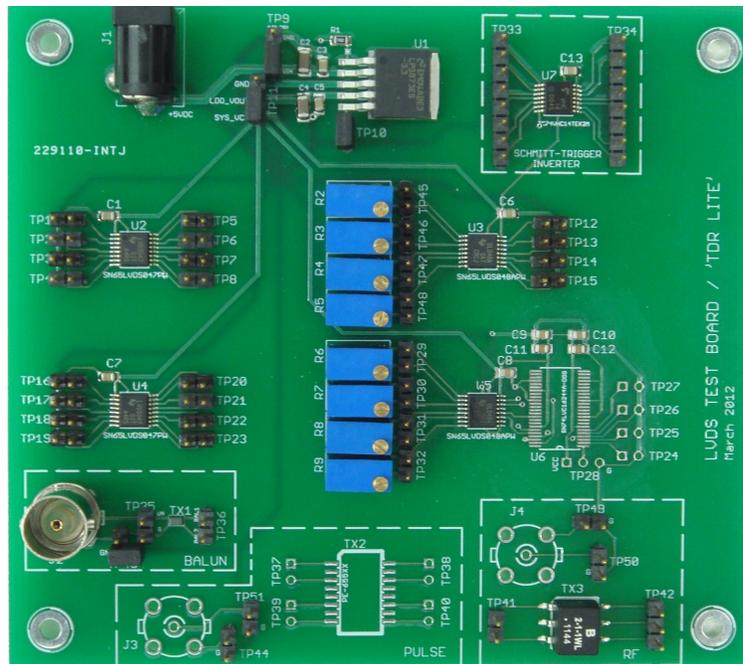
Figure 30: LVDS test board with TDR capabilities.
