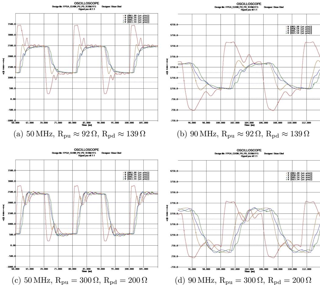
Figure 53: LineSim simulation of the FPGA\_CLKIN net at 50 MHz and 90 MHz using split end termination. The red trace is at the output of the LVDS reciever (U63, pin 10). The orange trace is at FPGA U58 pin 54, blue is at FPGA U41 pin 54, and green is at FPGA U13 pin 54.
