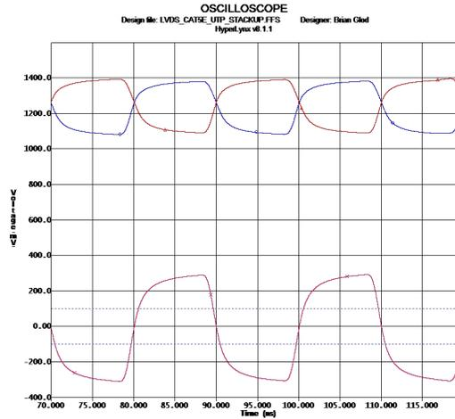
(b) Simulation of cat. 5e at 50 MHz
