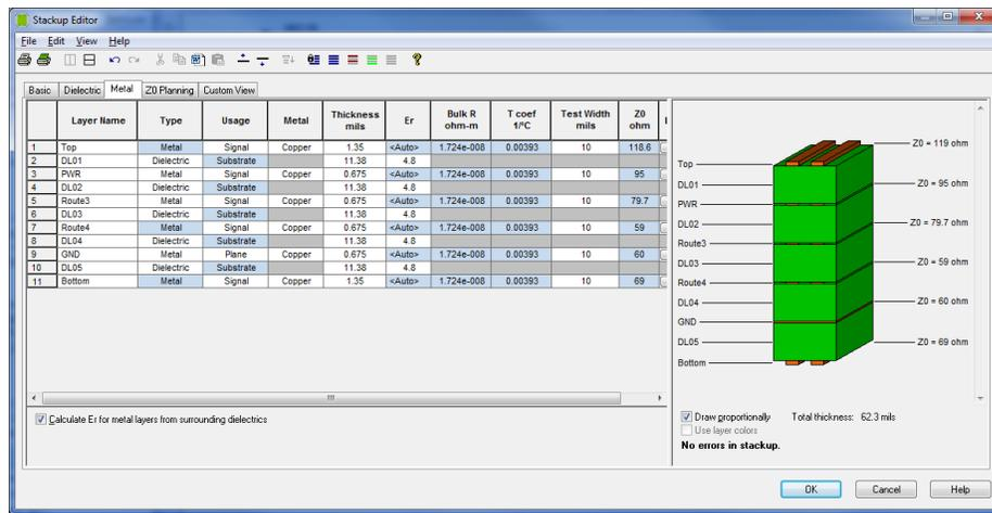
Figure 45: The fixed HyperLynx LineSim stackup of the CFB. Note the proper number of layers, layer thicknesses, and total board thickness.
