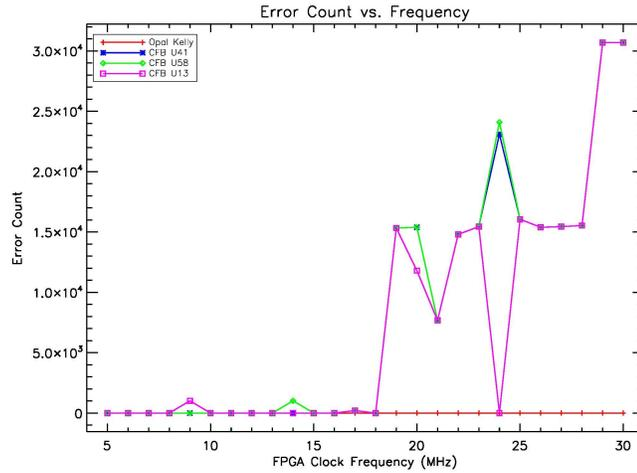
Figure 9: Initial bench-top CFB BER test results. The XEM3010 FPGA was directly controlling the CFB. This setup used the binary counter BER pattern from 5 MHz to 30 MHz with 1 MHz steps and 30 test iterations at each step.
