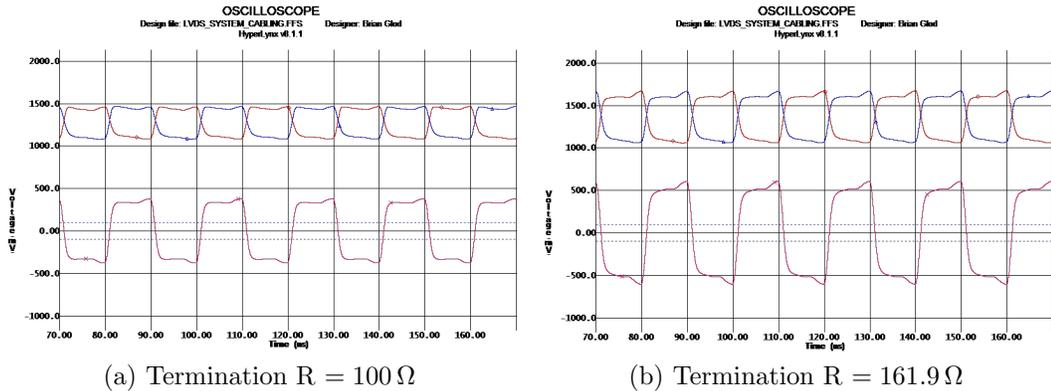
Figure 25: HyperLynx LineSim simulation of the system cables at 50 MHz. (a) Shows the resulting waveforms using  $100\ \Omega$  termination. (b) Shows the resulting waveforms using the optimal termination resistance of  $161.9\ \Omega$  as calculated by the HyperLynx termination wizard.
