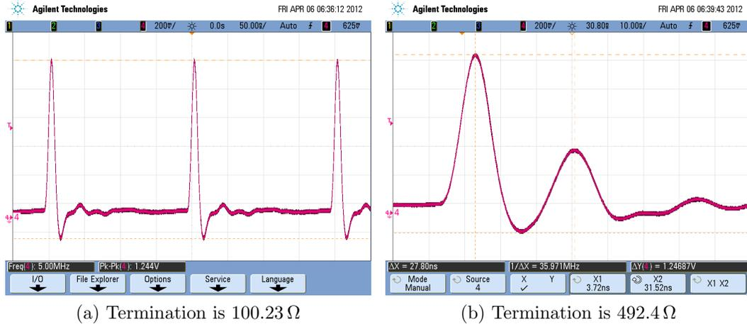
Figure 38: The oscilloscope capture in (a) shows no signal reflections, indicating proper termination; (b) shows a reflected pulse nearly 28 ns after the primary pulse. The reflection occurs because the termination resistance is not equal to the characteristic impedance of the cable.
