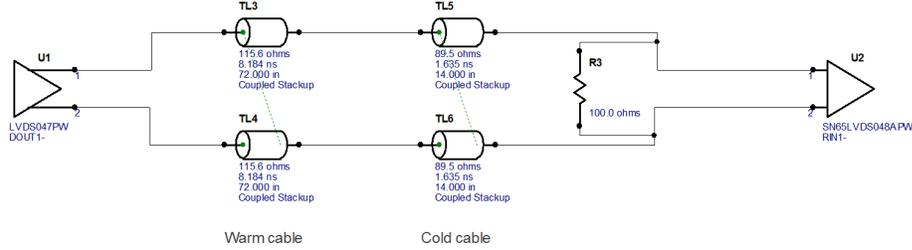
Figure 24: HyperLynx LineSim free-form schematic using system cable parameters.
