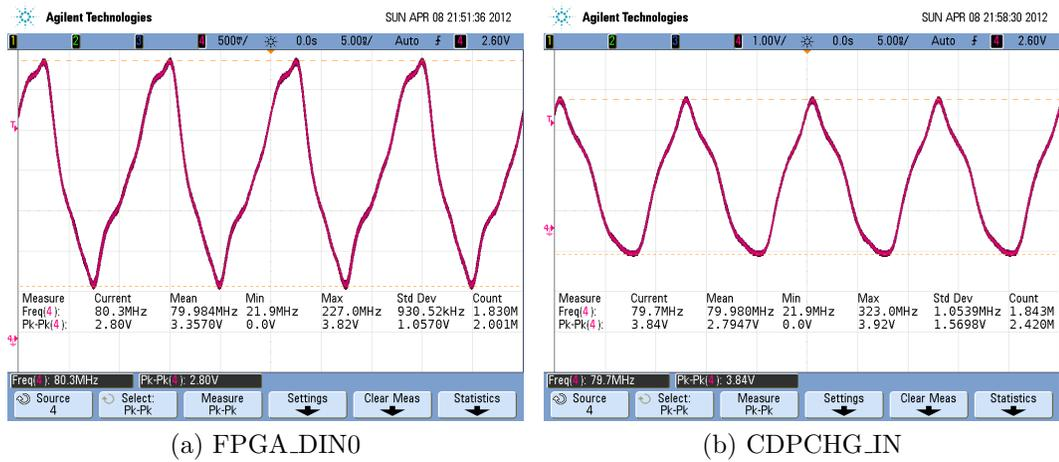
Figure 40: The output of the LVDS receiver when the input is terminated on the CFB. (a) Shows the FPGA\_DIN0 signal, and (b) shows the CDPCHG\_IN signal. Although not square waves, neither (a) nor (b) exhibit excessive ringback and are therefore superior to FPGA\_CLKIN.
