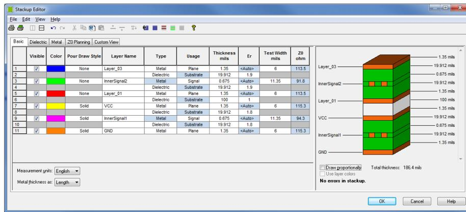
Figure 23: HyperLynx stackup using system cable parameters.
