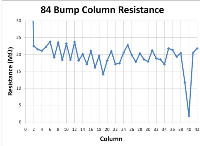
**Fig. 6.17** Measured resistance of columns of 84 bump bonds
