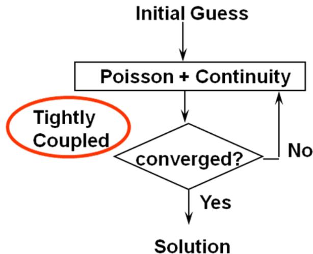
Fig. 3.5 Flow diagram for Newton method [24]
