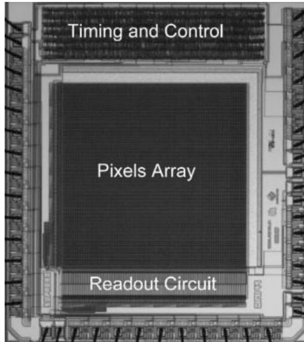
**Fig. 1.4** Typical monolithic CMOS image sensor [11]
