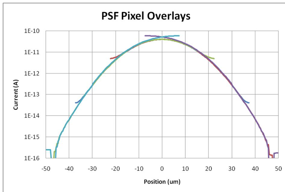
**Fig. 3.19** Current through pixels overlaid with maximums centered
