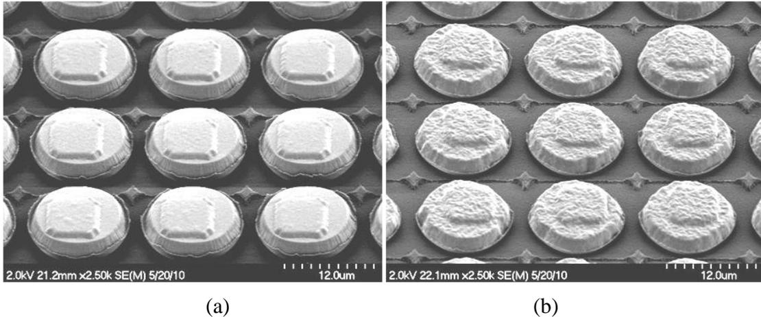
**Fig. 6.4** SEM of bump-bond array after lift-off (a) gold-tin(b) indium
