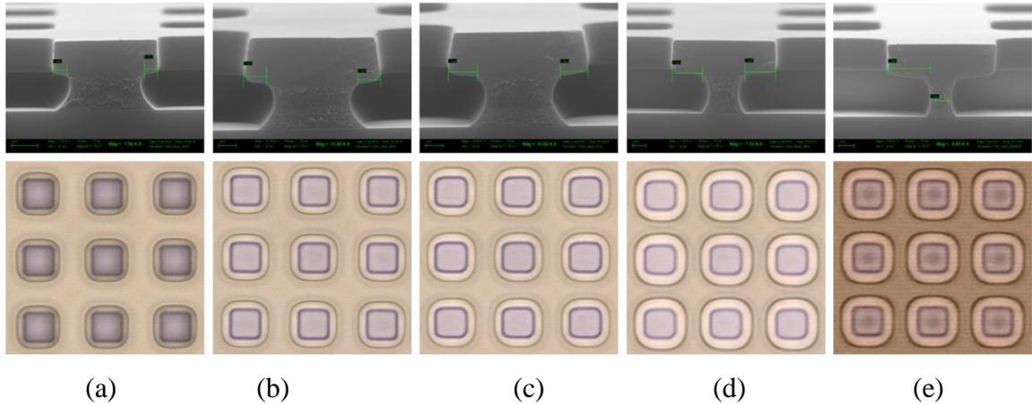
**Fig. 6.6** SEM cross-section and correlating optical micrograph of bump-bond opening in bi-layer resist stack for 190 C soft bake and development times of (a) 120 sec (b) 135 sec (c) 150 sec (d) 165 sec and (e) 180 sec
