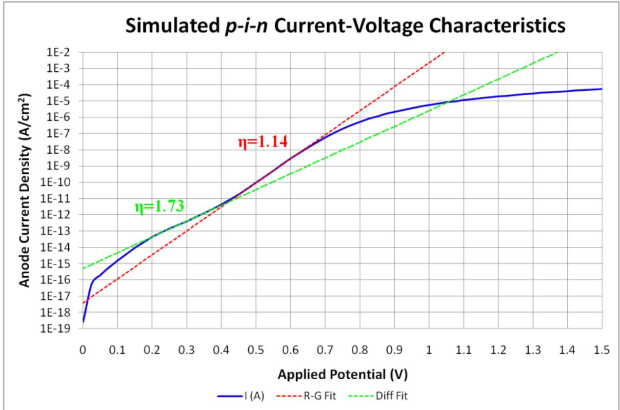
**Fig. 3.8** Simulated *p-i-n* diode forward bias current density
