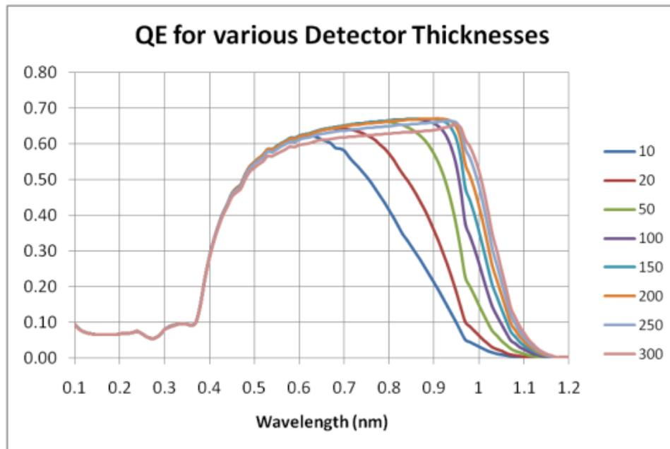
**Fig. 3.17** QE curves for detector thicknesses from 10 to 300 μm
