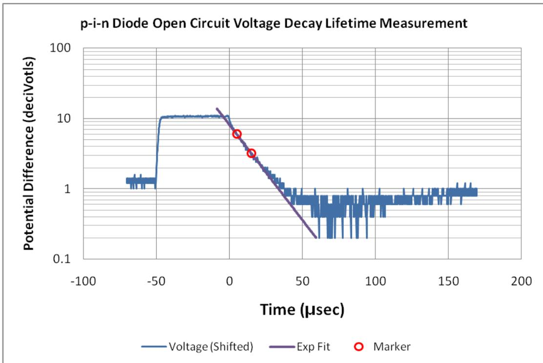
**Fig. 5.9** Diode junction voltage decay with exponential fit
