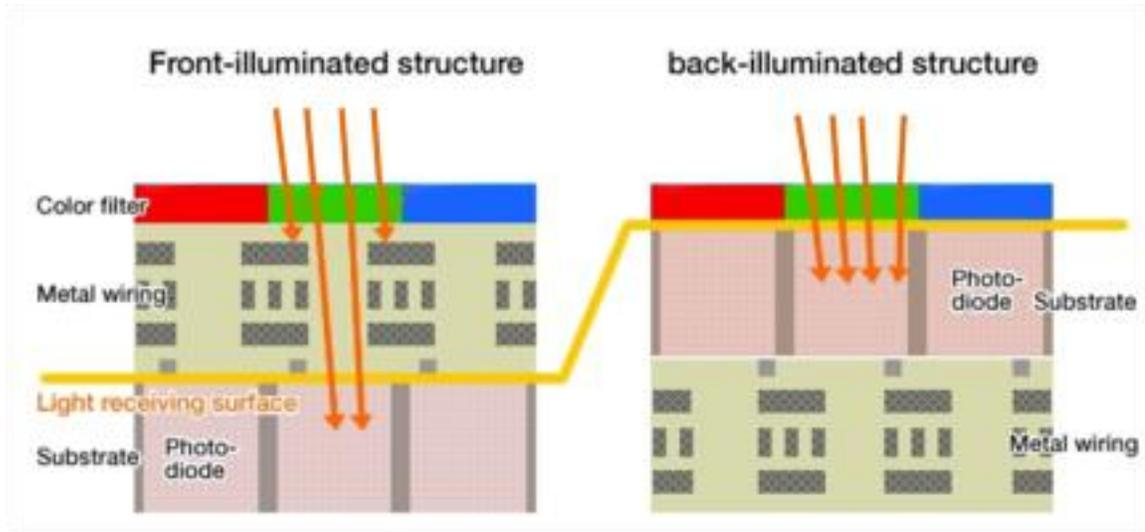
**Fig. 1.5** Schematic representation of front-side illumination (FSI) vs back-side illumination (BSI) [12]
