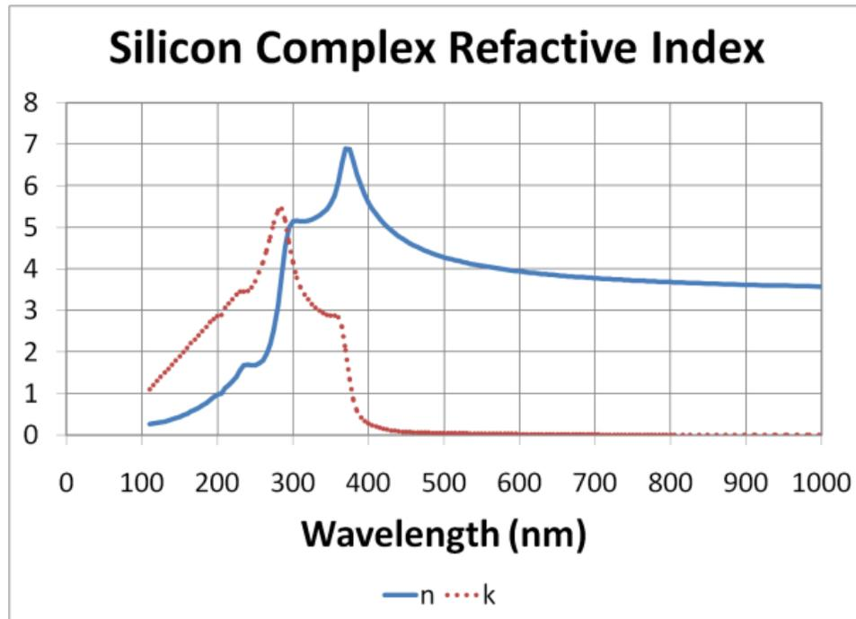
**Fig. 2.4** Complex refractive index vs. wavelength for silicon
