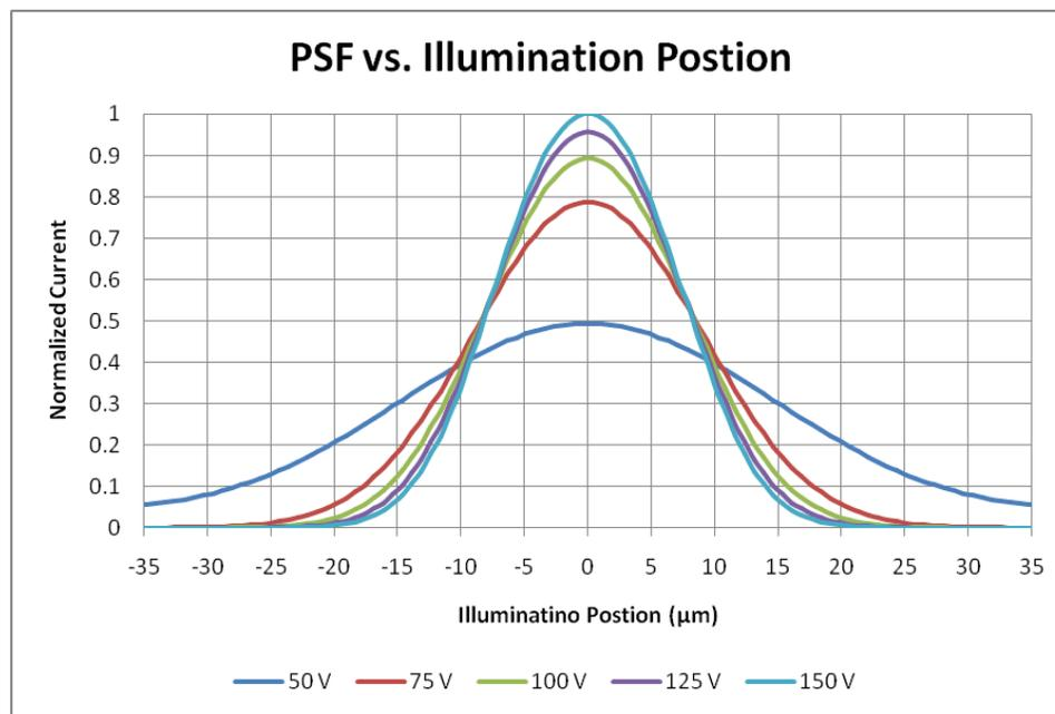
**Fig. 3.20** Simulated current vs. illumination position for 50, 75, 100, 125 & 150 V
