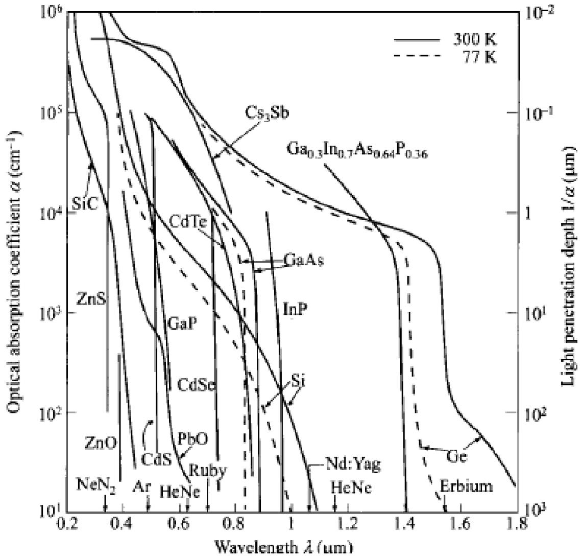
**Fig. 1.2** Optical absorption coefficients for various semiconductor materials [4]
