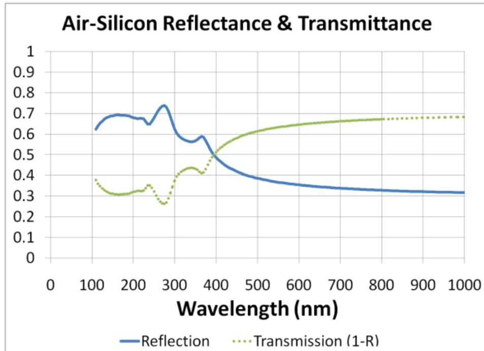
**Fig. 2.5** Reflectance and Transmittance at the air-silicon interface
