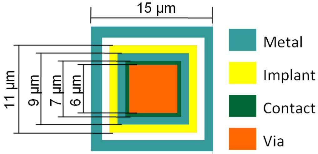
**Fig. 1.10** Pixel Design and Layout
