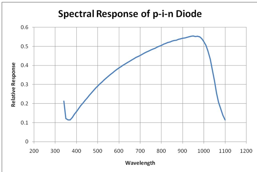
**Fig. 5.10** Short circuit spectral response of *p-i-n* diode
