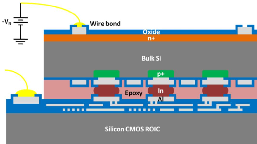
**Fig. 1.7** Illustration of Hybridized Image Detector cross-section
