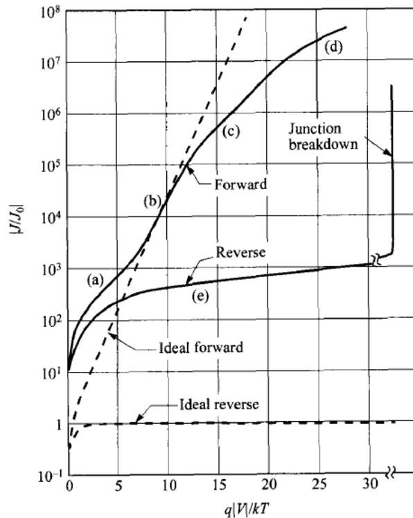
**Fig. 2.1** Current-voltage characteristics of a practical Si diode showing ideal and experimental behavior in forward and reverse modes of operation [4]
