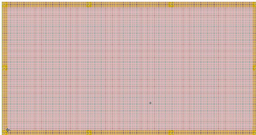
**Fig. 1.11** Layout of 256x128 p-i-n photodiode array with guard ring
