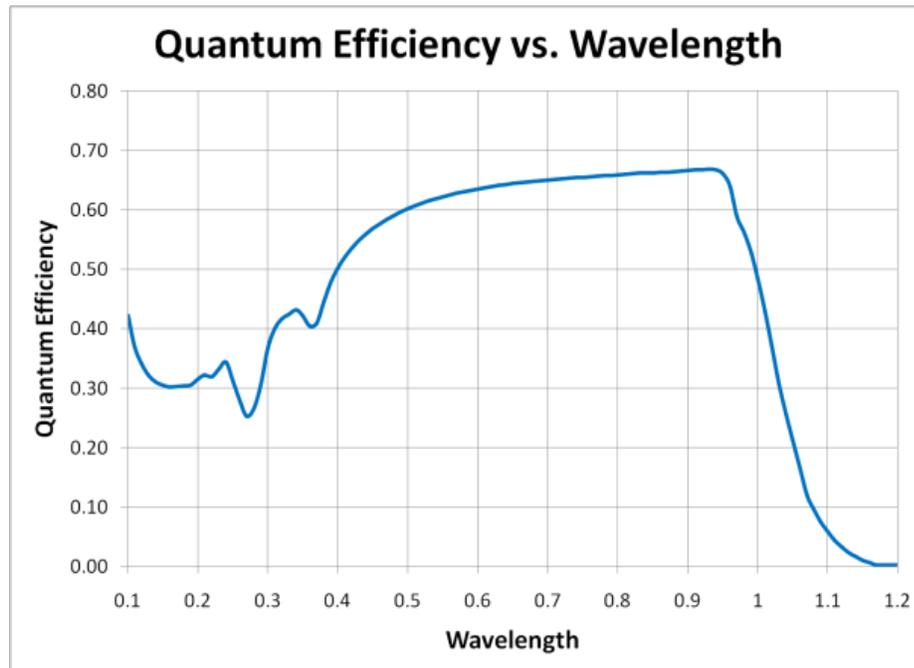
**Fig. 3.11** Typical quantum efficiency curve from SILVACO Atlas
