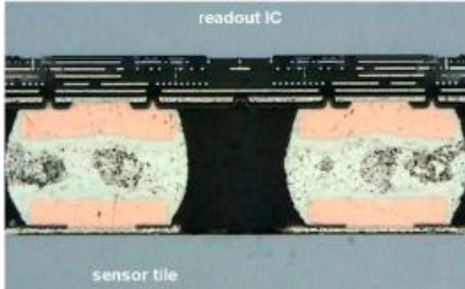
**Fig. 1.6** Cross-section of hybrid imager used in ATLAS detector [13]
