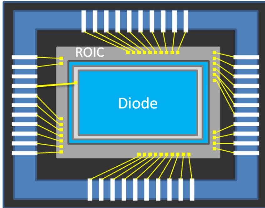
**Fig. 1.8** Top Down Illustration of Hybridized Image Detector
