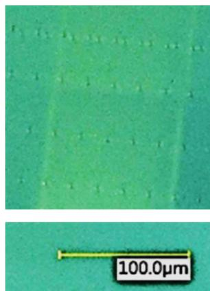
Fig. 13. Nanoindentation arrays on laser-processed spots, measured by Keyence microscope.
