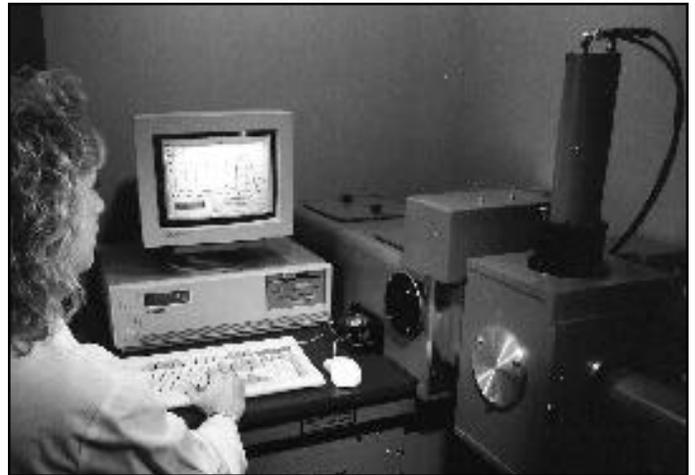
Critical coating performance is guaranteed by our ability to measure reflectance and transmittance using in-house state-of-the-art CAMS™ spectrophotometer systems.
