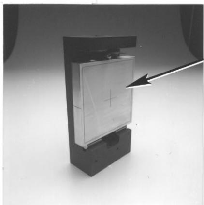
Grating Correctly Positioned in the Grating Holder
