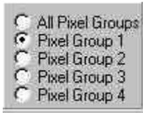
In the CCD peak monitoring mode it is possible to look at the data for an individual peak (pixel group) or all of the groups simultaneously.
