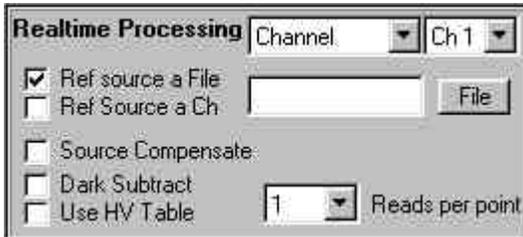
The Real Time Processing panel is used to define which detectors are to be read out for display and how the incoming data is to be processed before it is displayed. The top left choice field contains all of the display options available, which will vary depending on your system configuration. The typical choices are: Channel #, Chan #/reference, Channel #/ Channel #, Channel #/file, Absorbance, %Transmission, %Reflectance, and
