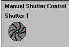
If a shutter is in the system and the light path includes a single channel detector, the manual shutter control panel will appear. Click on the shutter icon to open or close the shutter. The current status of the shutter is shown by the icon (closed in this illustration).
