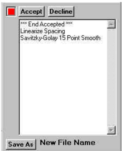
The manipulations log panel keeps track of every operation performed on the spectrum. Each operation or series of operations can be accepted or declined by clicking on the appropriate button. If you wish to save the treated spectrum, click on the Save As button. The save file as dialog box will appear. All of the operations performed on the spectrum and the date they were performed are saved in the new data file's header.
