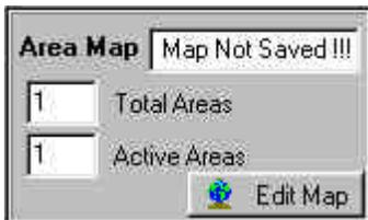
If a CCD is in the light path, the area map information panel will appear. It shows the name of a stored map if loaded, in the top field, the total number of areas created on the chip and how many of these areas are going to be actively read out. Clicking on the Edit Map button brings you to the map creation panel in the survey screen.
