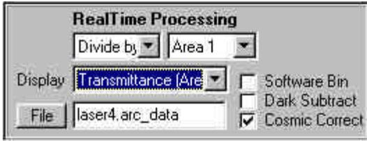
The CCD real time processing panel shows how the incoming data is being treated before presentation on the screen. The top left dialog box has three options; no op, subtract, and divide by one of the areas that are being readout on each acquisition. The area number to be subtracted or to be the divisor is selected from the right drop down field. The data can be displayed in raw
