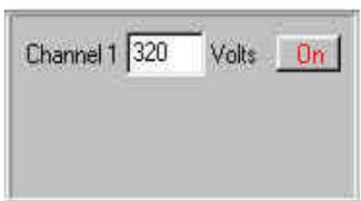
The High Voltage panel will appear if there are photomultiplier tubes in your system. The current value is that last used in the Survey mode. You may change the high voltage by highlighting the field and entering a new value. A set button will appear to validate the change. If a stored routine is loaded, the high voltage will be changed to the value stored in the routine. You can turn the high voltage on or off by clicking on the On/Off button.
