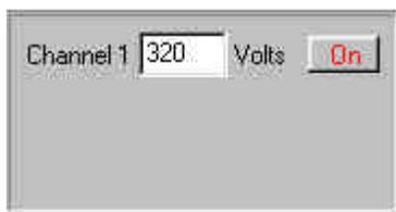
The High Voltage panel will appear if there are photomultiplier tubes in your system. The current value is what was last used in the Survey mode. You may change the high voltage by highlighting the field and entering a new value. A set button will appear to validate the change. If a stored routine is loaded the high voltage will be changed to the value stored in the routine. You can turn the high voltage on or off by clicking on the On/Off button.
