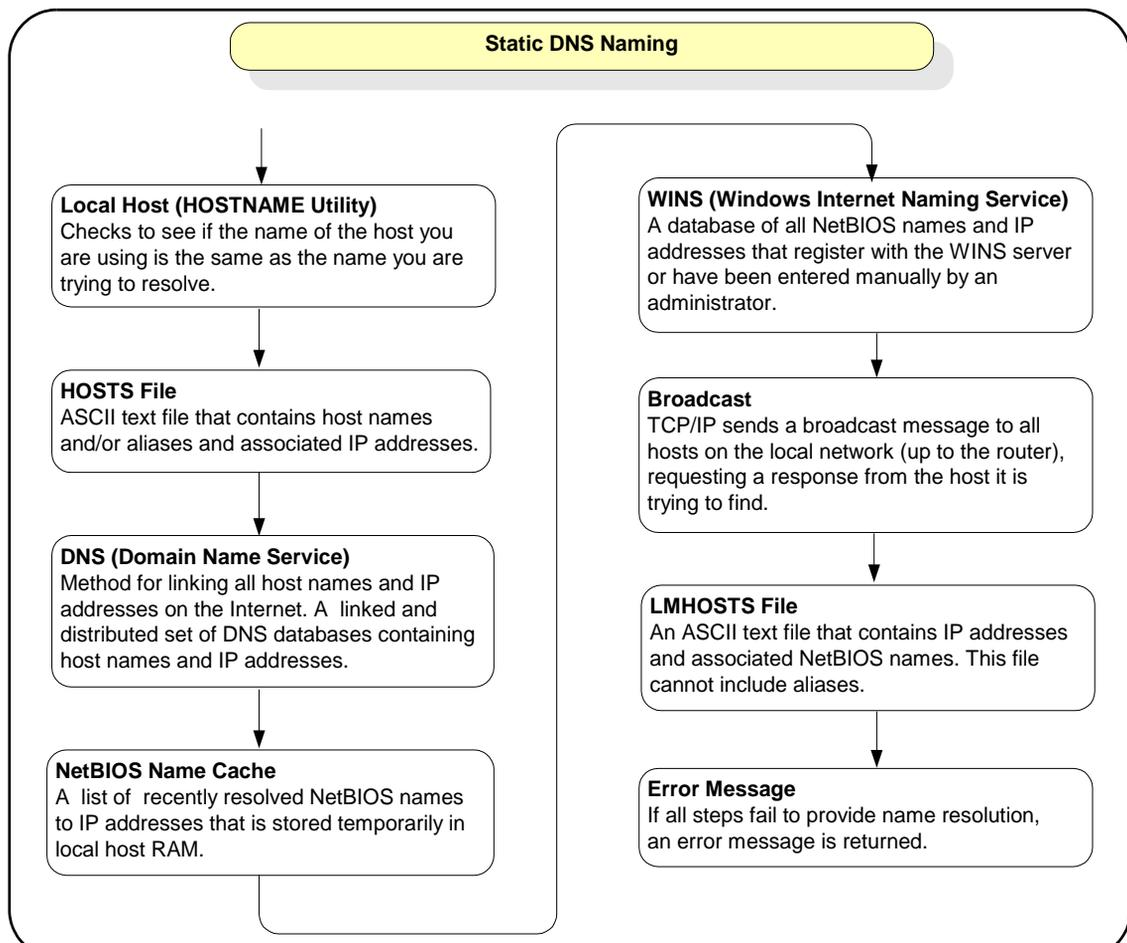
Figure 65 Static DNS Naming
