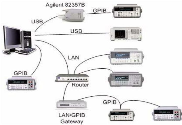
**Figure 1** Example test system: PC, instruments, Three Types of I/O
