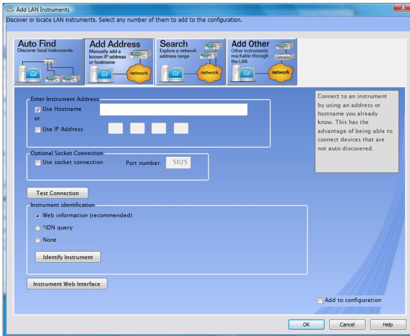
**Figure 32** Add LAN Instruments Add Address Dialog screen
