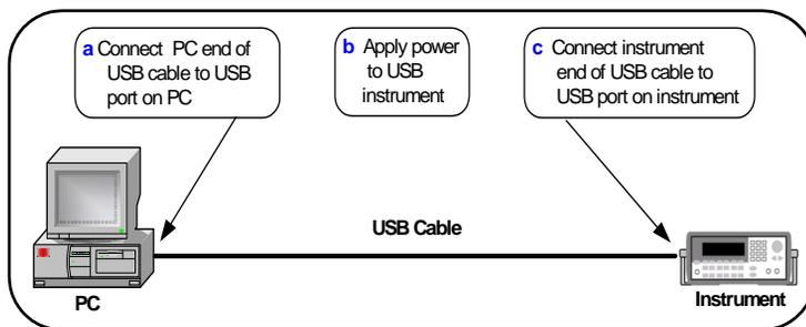
**Figure 18** Connecting a USB Instrument to a PC
