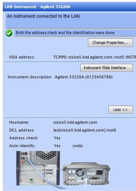
**Figure 45** LAN Interface Configuration Dialog Box
