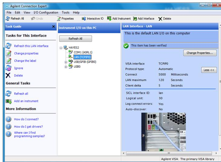
**Figure 30** Agilent Connection Expert, LAN Connections
