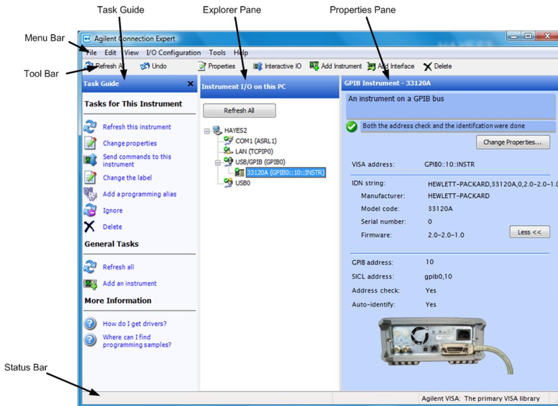
Figure 2 Agilent Connection Expert Screen
