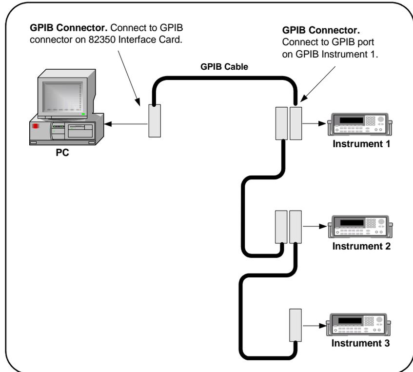
**Figure 12** Connecting Three GPIB Instruments
