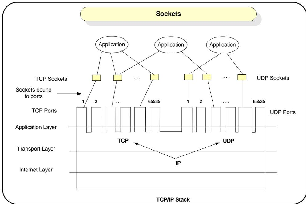
**Figure 61** Typical Socket Architecture
