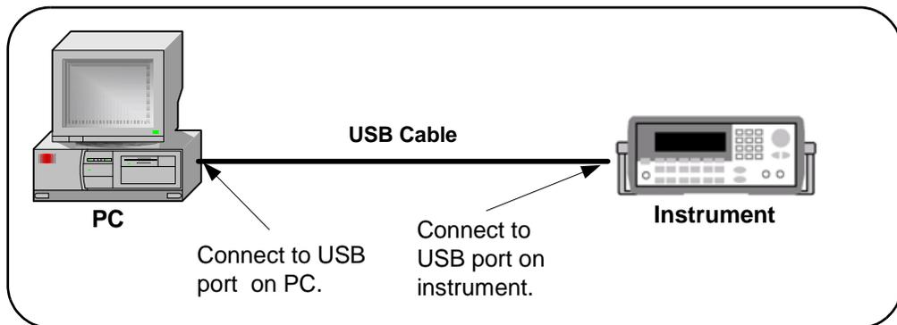
**Figure 17** Typical USB Interface System
