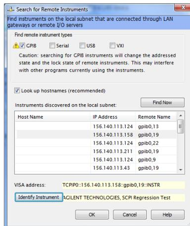
**Figure 38** Discovery of LAN Instruments on the Subnet
