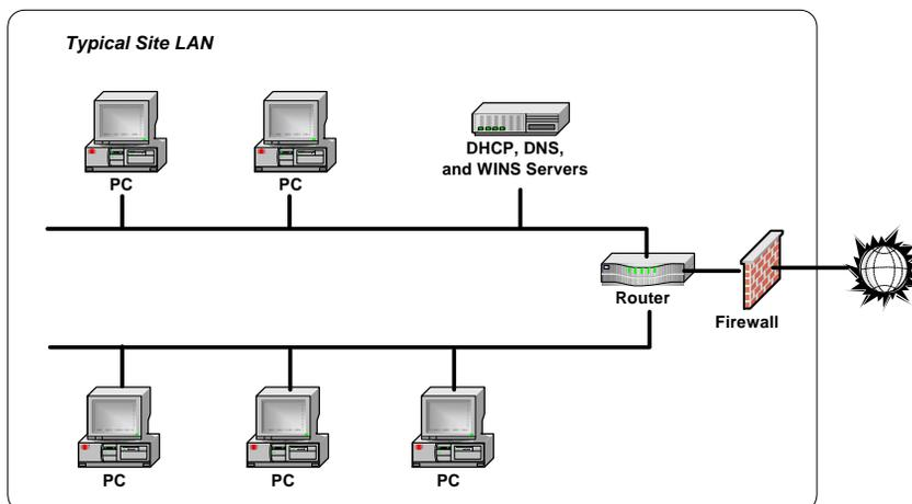
**Figure 53** Portion of a Typical Site LAN
