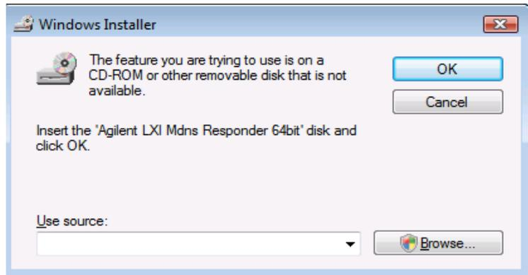
If you see this dialog box, insert the *Automation-Ready CD with Agilent IO Libraries Suite* into the CD-ROM drive of your PC. Windows will use the files on the CD to make repairs.
