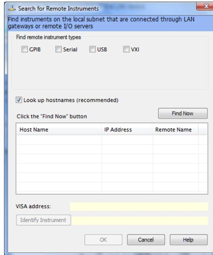
**Figure 37** Search for Instruments on the LAN Dialog Box
