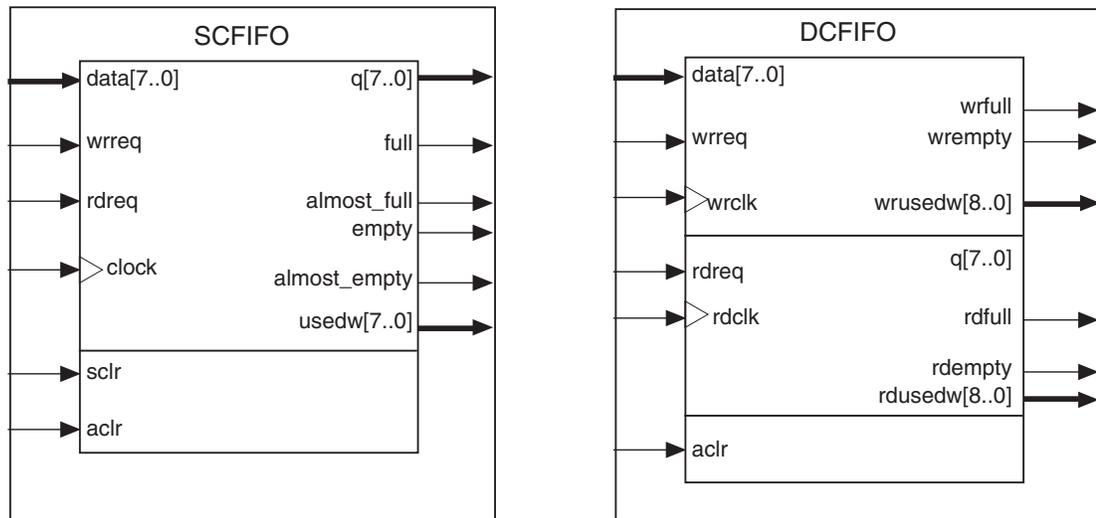
For the SCFIFO, the read and write signals are synchronized to the same clock, while for the DCFIFO, the read and write signals are synchronized to the `rdclk` and `wrclk` clocks respectively. The prefix `wr` and `rd` represent the signals that are synchronized by the `wrclk` and `rdclk` clocks respectively.
