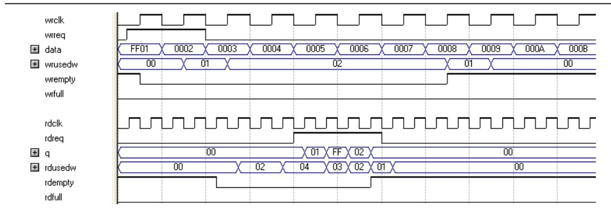
In this example, the read port is operating at twice the frequency of the write port. Writing two 16-bit words to the FIFO buffer increases the wrusedw flag to two and the rusedw flag to four. Four 8-bit read operations empty the FIFO buffer. The read begins with the least-significant 8 bits from the 16-bit word written followed by the most-significant 8 bits.
