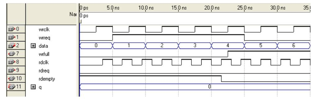
Figure 3 shows the functional timing requirement for the rdreq signal with respect to the rdempty signal.
