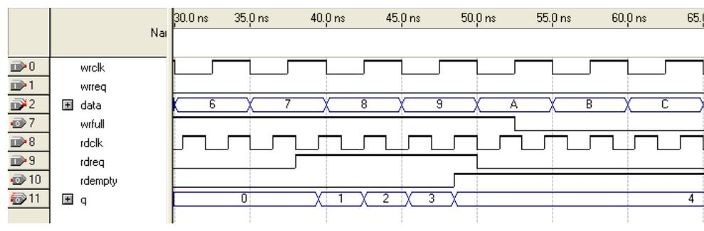
The required functional timing for the DCFIFO as described previously is also applied to the SCFIFO. The difference between the two modes is that for the SCFIFO, the wrreq signal is with respect to full flag and the rdreq signal is with respect to the empty flag.
