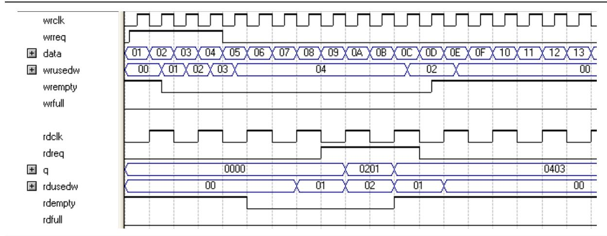
In this example, the read port is operating at half the frequency of the write port. Writing four 8-bit words to the FIFO buffer increases the wrusedw flag to four and the rusedw flag to two. Two 16-bit read operations empty the FIFO. The first and second 8-bit word written are equivalent to the LSB and MSB of the 16-bit output words, respectively. The rdempty signal stays asserted until enough words have been written on the narrow write port to fill an entire word on the wide read port.
