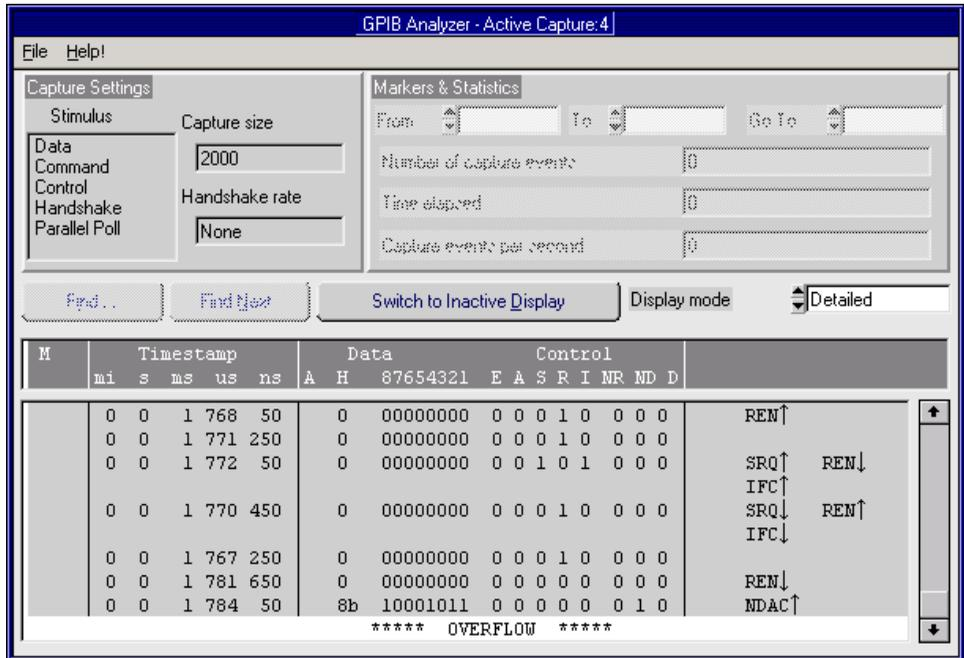
Figure 3-1. Overflow Error
