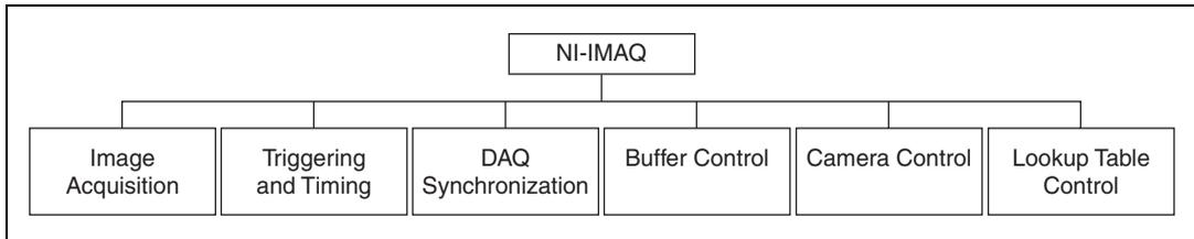
**Figure 1-2.** NI-IMAQ Functions
