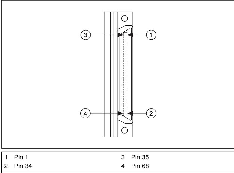
**Figure 2.** 68-Pin VHDCI Connector (Cable)
