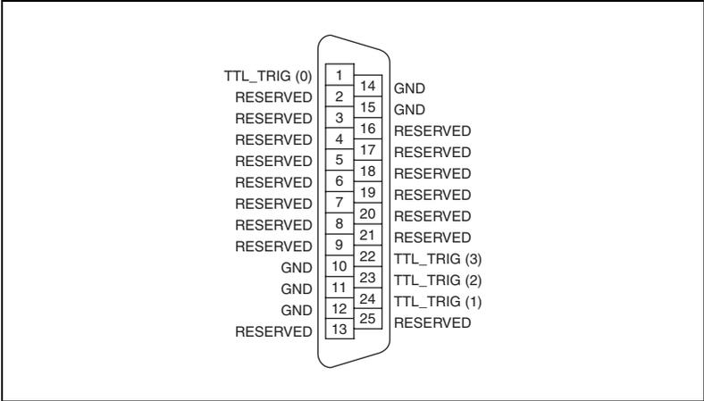
Figure 5. 25-Pin D-SUB Trigger Connector Pinout (Cable)
