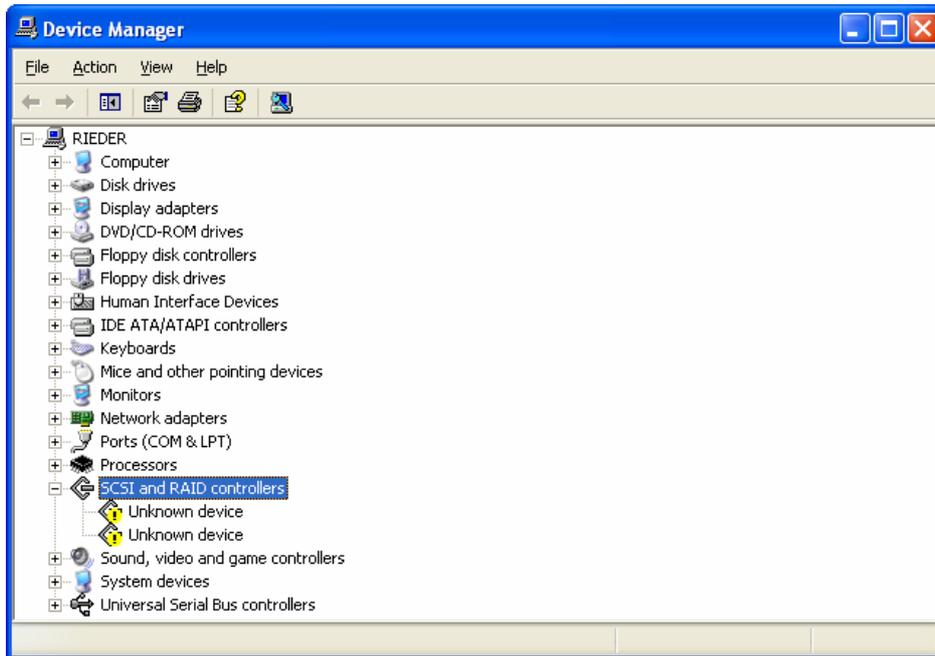
Right click on the desired Host Bus Adapter and select “Update Driver...”. Make sure the installation CD-ROM is in the CD drive and select “Install the software automatically (Recommended)”. Press “Next” to install the software.
