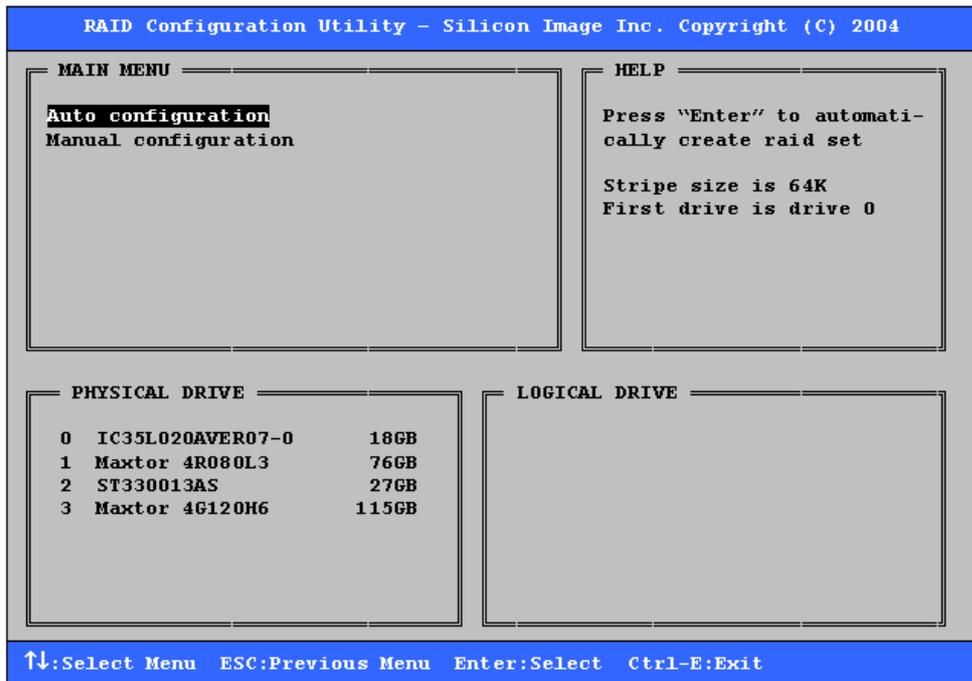
4. If manual configuration is selected, the chunk size of Striped Sets can be selected. For Mirrored Sets, the Source and Target drives can be selected.
