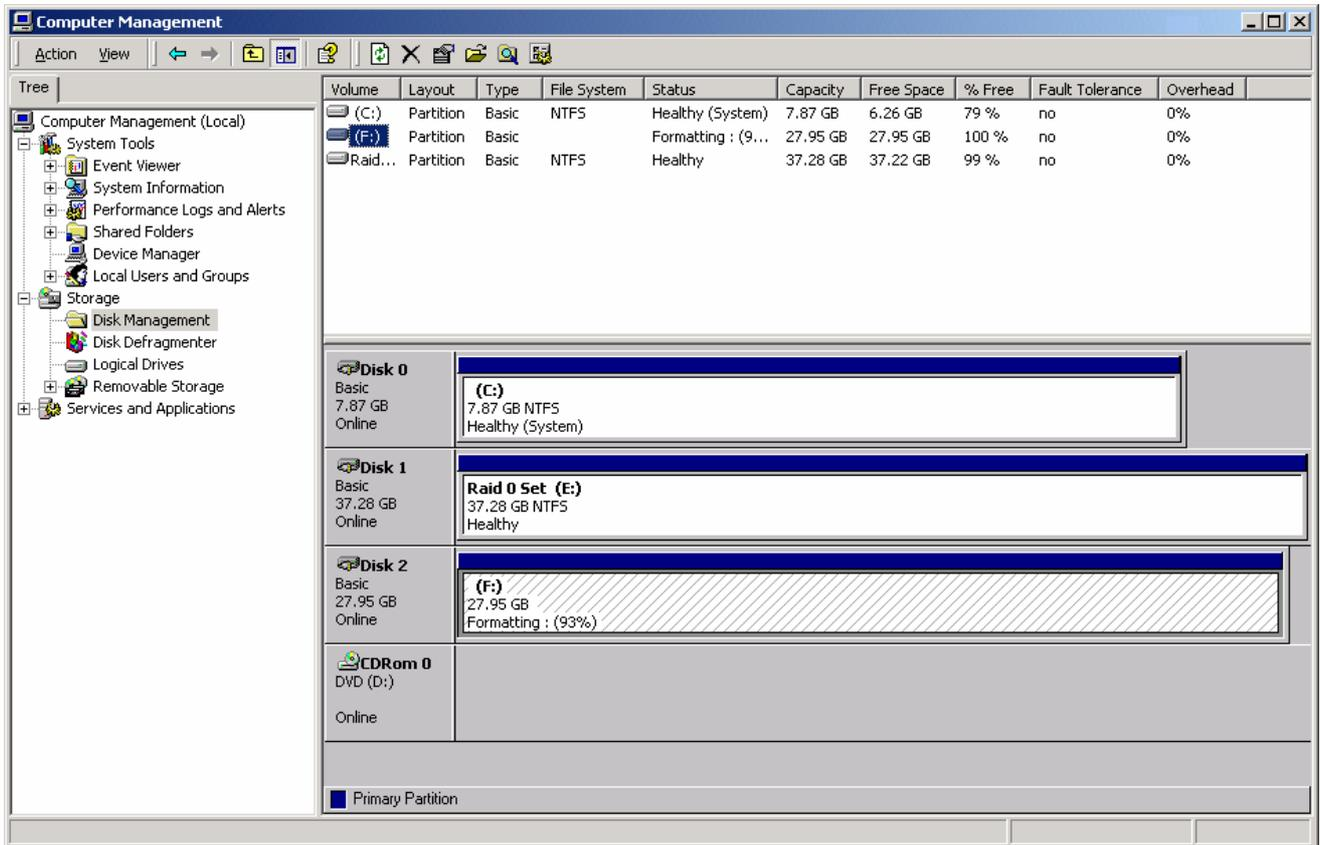
Repeat the above procedure as needed for any other partitions. Close the Data Management window by clicking on the small boxed "X" in the top right corner of the window. Click on the "My Computer" icon on the Desktop. The new drives will be visible and properly named. The new disks are available for use.
