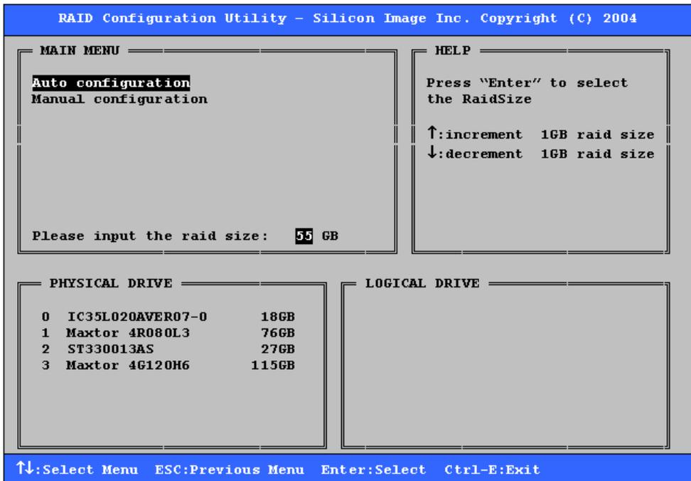
7. After the RAID set size is set, the message "Are You Sure?" will display before completing the configuration. Answer "N" to abort the creation of the new RAID set, or "Y" to proceed with the RAID set creation.
