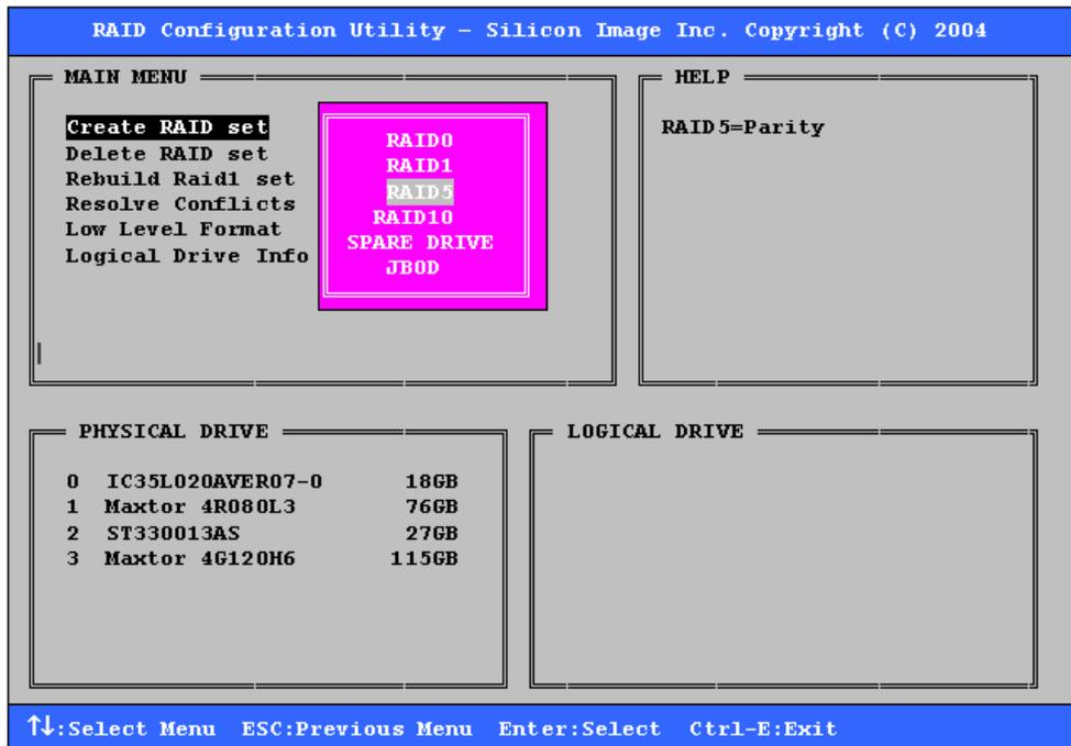
3. Select Automatically or Manually configuration of the RAID Set.
