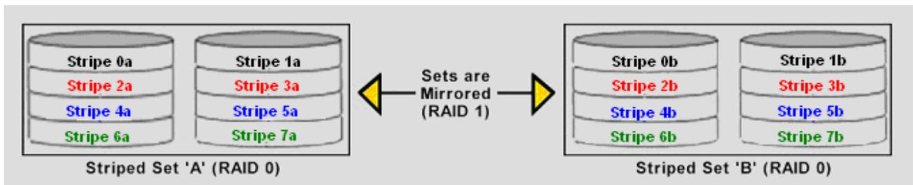
The data is written to RAID Group A, which is striped (RAID 0). This allows maximum speed. The data is then mirrored to another RAID 0 striped set, which is Set B in the figure above. This provides data redundancy (RAID 1), and thus increased data security.
