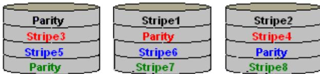
Parity RAID uses less capacity for protection and is the preferred method to reduce the cost per megabyte for larger installations. Mirroring requires 100% increase in capacity to protect the data whereas the above example only requires a 50% increase. The required capacity decreases as the number of disks in the group increases.
