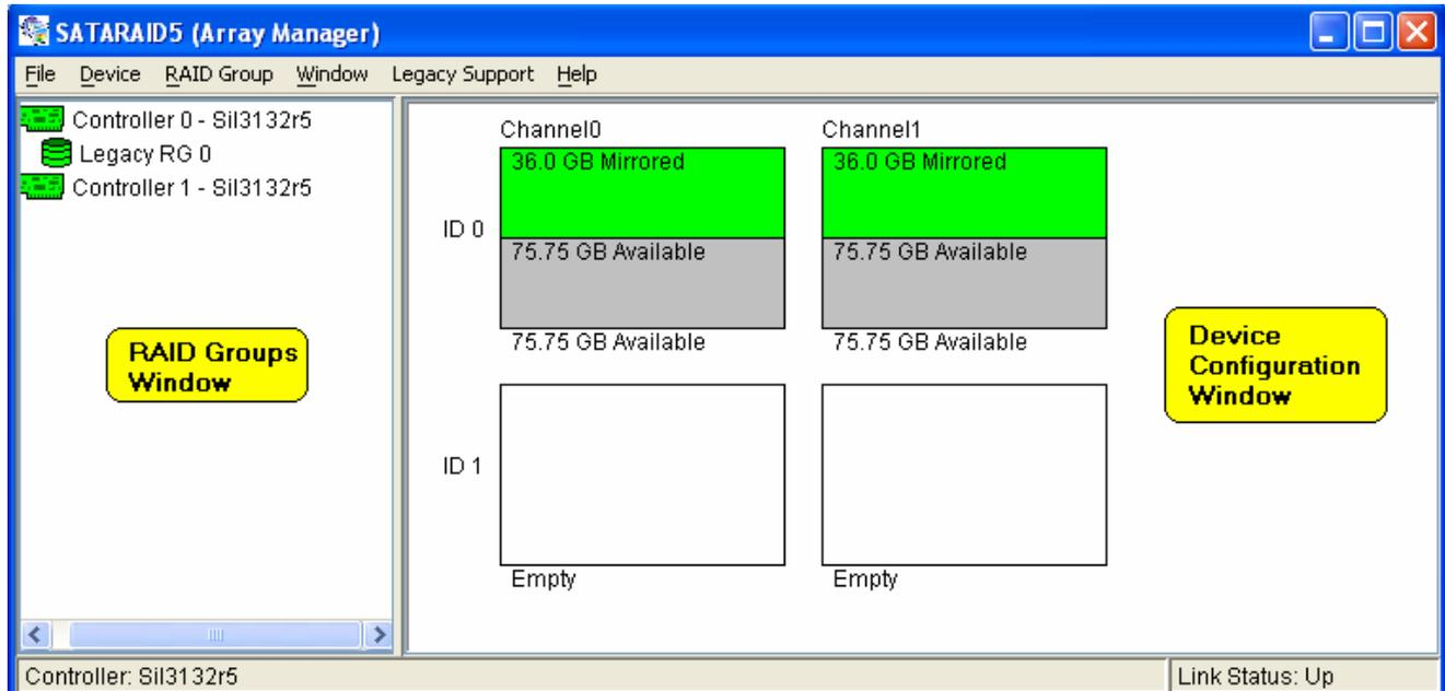
The RAID Groups window identifies SATA host adapters and configured RAID groups. For systems with more than one Silicon Image Host Bus Adapter installed, you can switch between cards by selecting the desired card in the RAID Groups Window.
